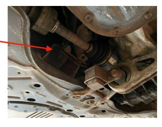
Use the supplied M10 lock washers and nuts to secure the front plate into place. You can gain access by turning the tire out and reaching through the spot outlined.
