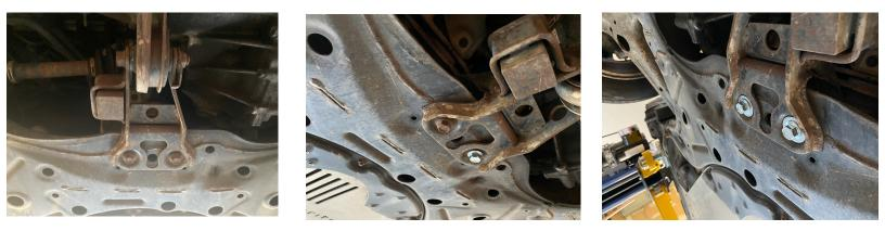
STEP 1: There are two bolts in the rear engine mount. Remove one bolt at a time and replace with the M10 x 80 flange supplied in the hardware kit.
