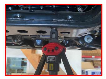
In this part of the installation process, we recommend using a rivet nut installation tool.
