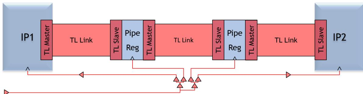
Figure 4 – Pipelined TileLink.
