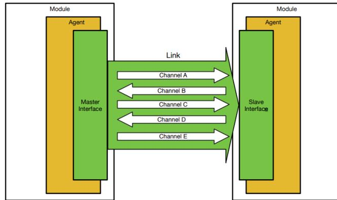
*Figure 2 – The five channels of a TileLink.*
