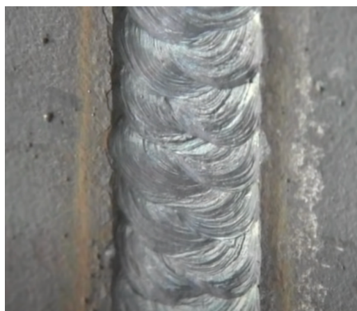
Figure 5. The weld bead produced by the weave bead technique shown in Figure 4 (Collier, 2015, 4:10). The side by side, overlapping crescent-shaped ripples result from weld puddles freezing on each side of the weld bead.
