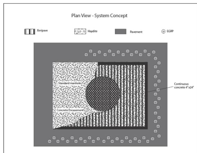
storm drain is stored in the pervious pavers and porous aggregate and ultimately infiltrated using EGRP® to rapidly incorporate the stored volume into the native soils.
