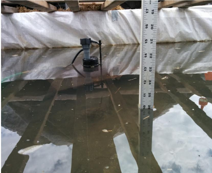
Figure 26. Float valve (background) and water level gauge.
