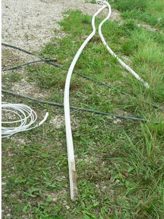
*Figure 16. 20-ft. EGRP nest showing sampling tube "screen."*
