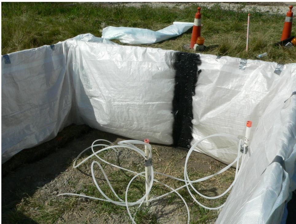
*Figure 20. Pool wall assembly wrapped in 0.024-inch rip-stop poly sheeting and sealed with commercial waterproofing spray (black stripe).*
