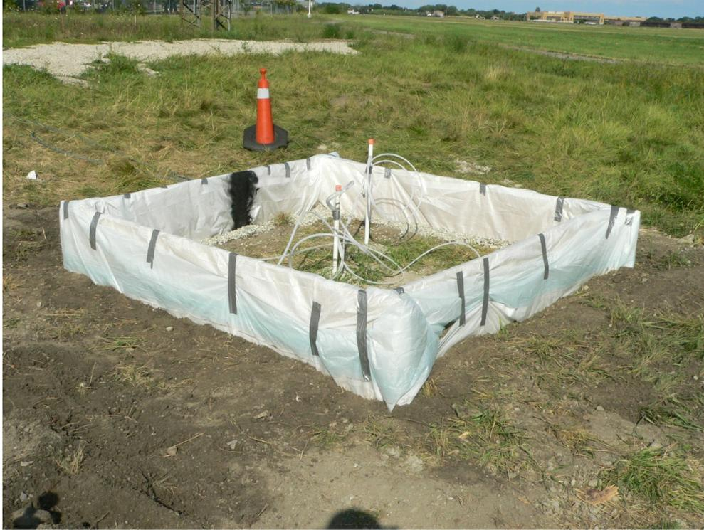
*Figure 21. Infiltration pool walls installed in the trench, exposing 1.5 feet above grade.*
