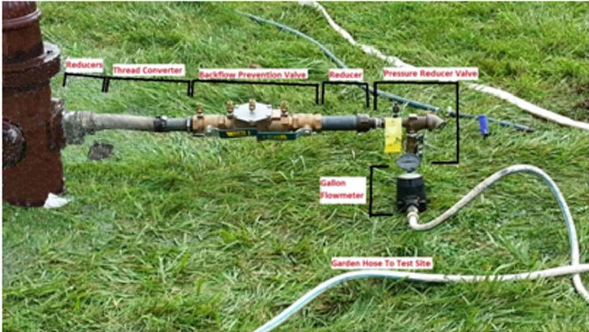
*Figure 24. Hydrant hardware necessary to reduce the pressure, prevent backflow and step-down the thread size to accommodate a standard garden hose connection.*
