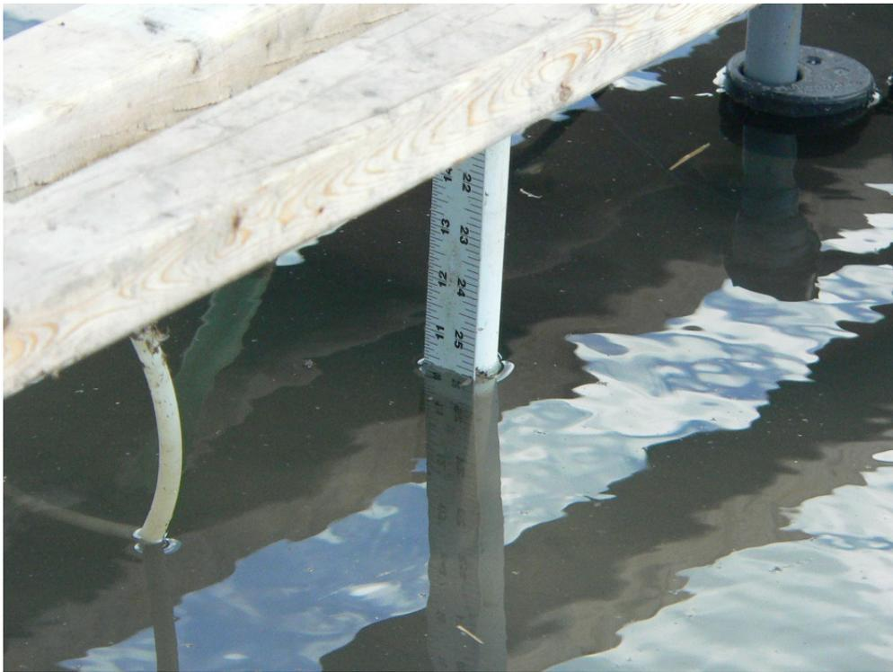
Figure 30. Second slug test filled the pool to 7 3/8" [10 3/8" on staff gauge] with 41.0 mg/L Br<sup>-</sup> water.
