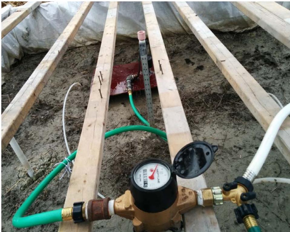
Figure 27. Totalizing flow meter connected to the infill hose (white). The green hose in the lower-right of the picture provided hydrant water for filling the 250-gallon poly tank used to mix the tracer slug (note the valves which allowed the poly tank to be filled without the water running through the totalizing flow meter).
