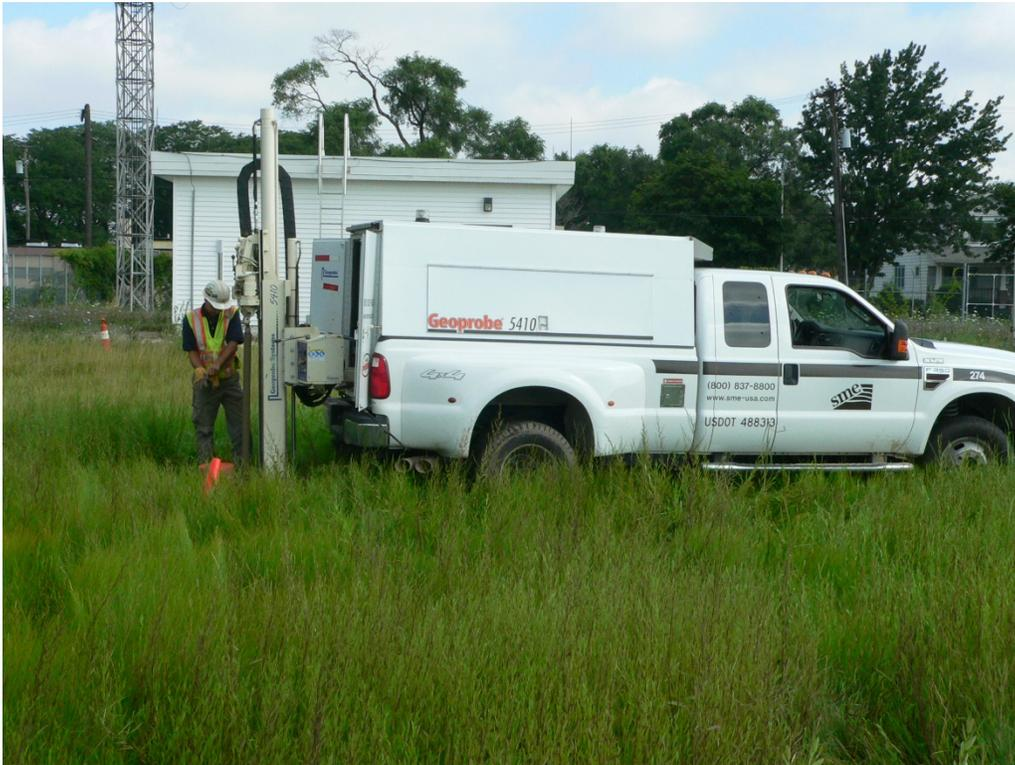
Figure 4. Truck-mounted GeoProbe® taking continuous soil cores at the site.
