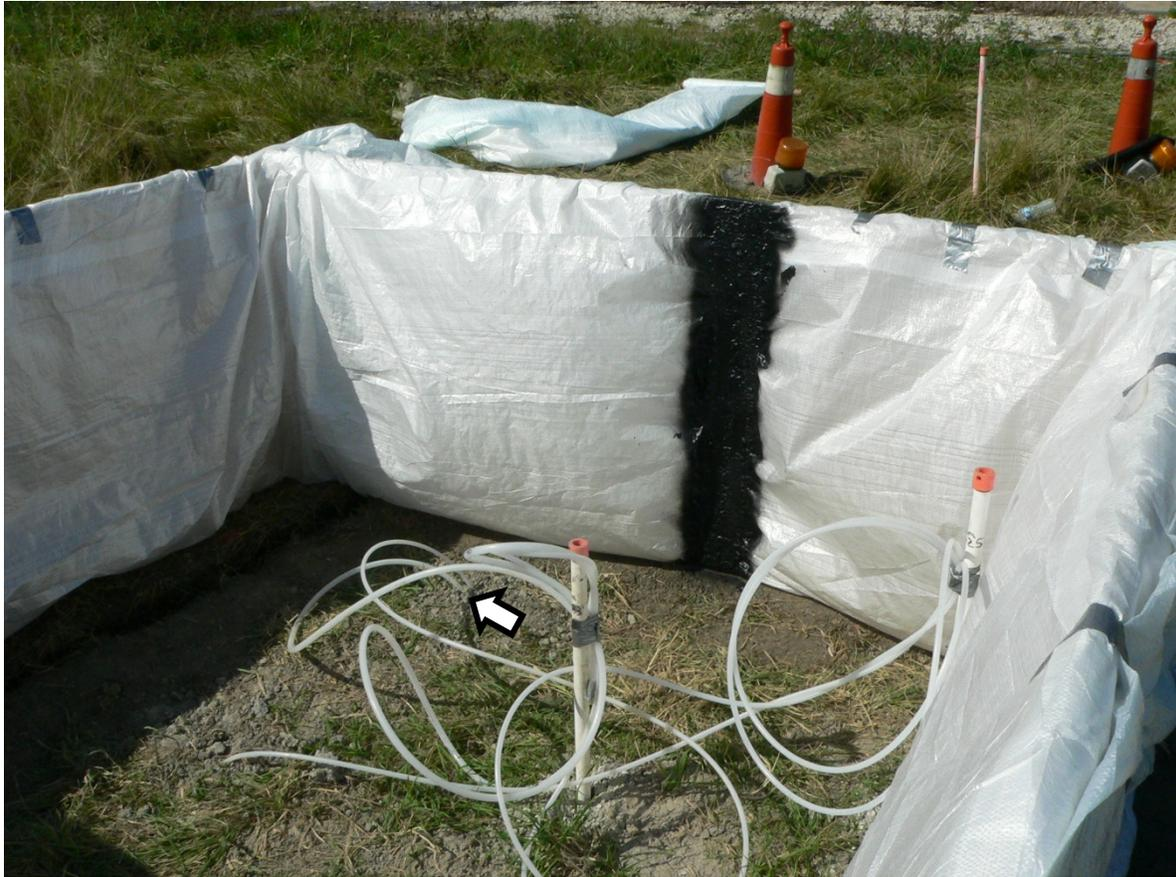
Figure 18. EGRP nest sampling tubes extended above grade to facilitate sample collection. The arrow points out the 40-ft. EGRP nest that has two sampling tubes, one at a depth of 20 feet and a second at a depth of 40 feet.
