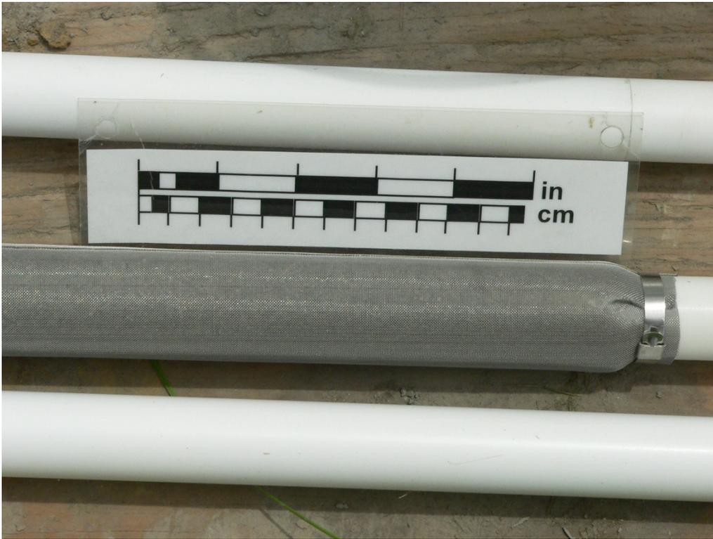
Figure 9. Close-up of sand-pre-packed screen with 10-slot mesh.
