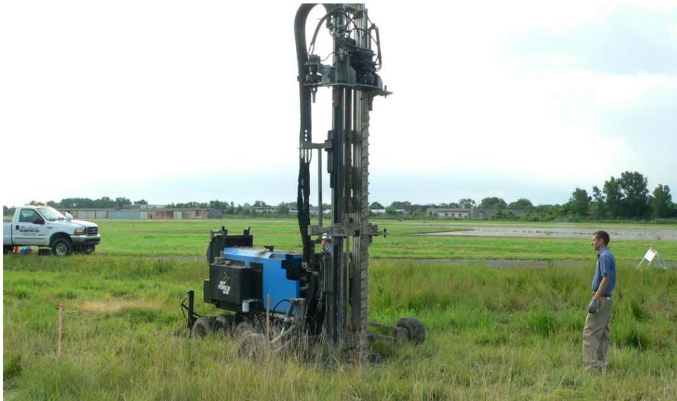
*Figure 6. Parjana's custom, self-propelled, auger drill rig.*
