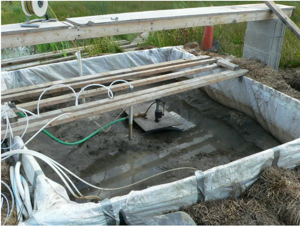
Figure 29. Infiltration pool pumped nearly dry in preparation for the second slug test.
