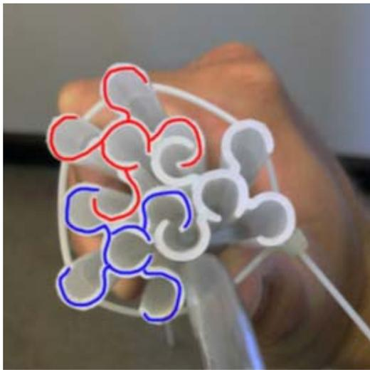
*Figure 12. EGRP nest composed of three individual EGRPs (colored for clarity) and a sampling tube zip-tied together.*
