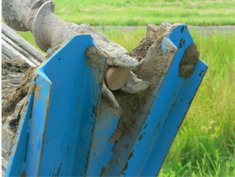
*Figure 7. Hollow-stem auger with drilling plug installed.*
