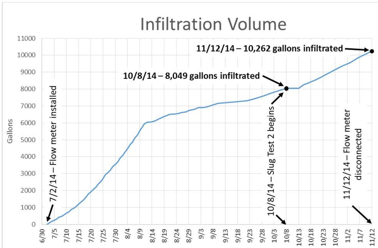
Figure 28. Total hydrant water infiltration measured by the flow meter.
