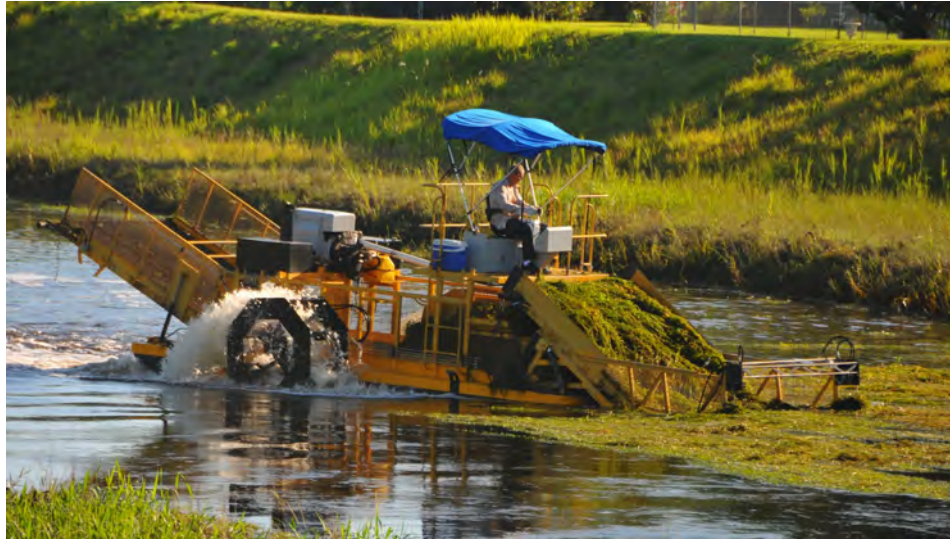
Fig. 39. Mechanical harvester removing nuisance plants.
