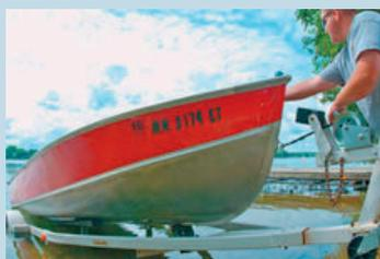
One person should be able to competently back the trailer down the ramp and unhook, while another fires it and pulls it clear of the trailer. Don't unhook the bow line until the engine is running, in case of a problem. After you launch, wait til your driver returns and then
