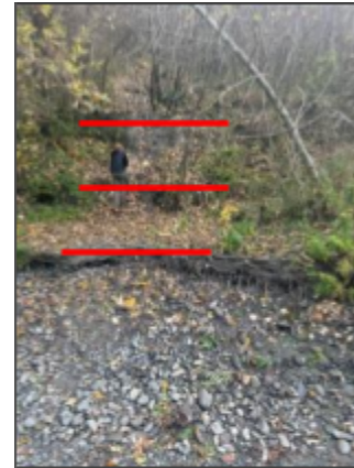
Figure 5. Picture taken from previous site of lake Aldwell. The red lines show layers of sediment. Jeron for scale.
