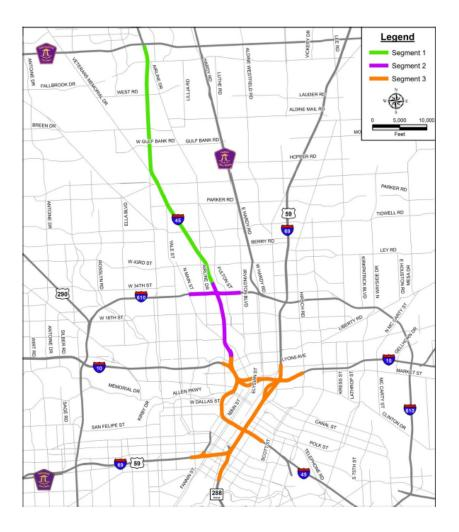
46. <u>Segment 1 (Green)</u>: Segment 1 widens the existing I-45 primarily on the west side of the roadway, which requires about 200 to 225 feet of new right-of-way ("ROW"). A new ROW on the east side is also required in part of Segment 1 between Crosstimbers Street and I-610. Thus, the total new ROW required for Segment 1 is about 246 acres.
