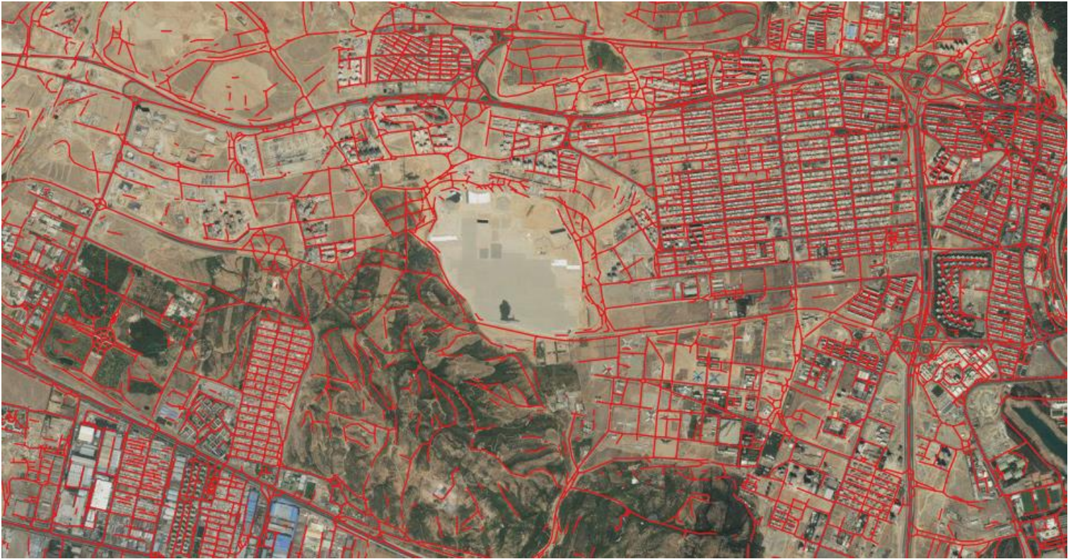
Figure 8: Single time period results from Orbital Insight's land use algorithm, showing specifically a roads-as-linestrings output class across a mixed urban/unpopulated area and challenging arid/desert conditions. These results are also based on medium-resolution imagery (Planet, 3–5m GSD), visualized over generic/older basemap imagery.
