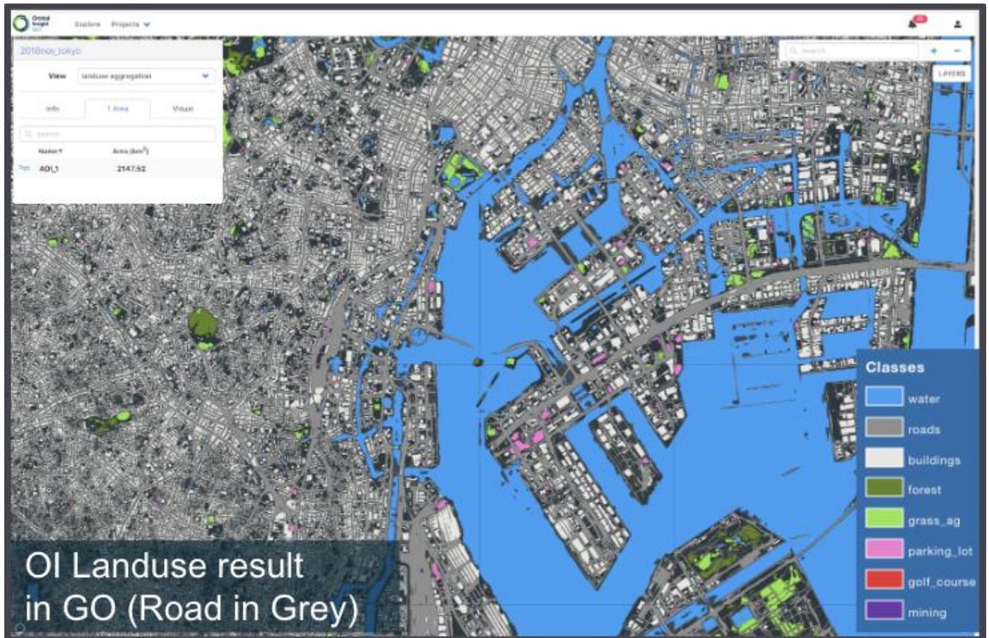
Figure 7: Single time period results from Orbital Insight's land use algorithm, applied across an entire city scale, and based on medium-resolution imagery (Planet, 3–5m GSD).
