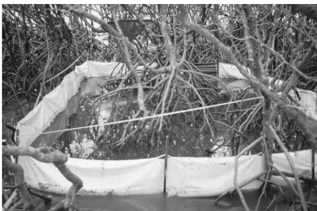
Fig. 2 One of 18 experimental enclosures where oil treatments were applied to plots of mature Rhizophora forest. Plots were located within the forested area, approximately 50 m from the sea edge (in the background of the photo). The image was taken immediately after oiling so oil can be seen on the inner sides of enclosure panels. Enclosures were open to tidal flows through a 'tide gate' (the darker panel on the far side) which allowed relatively normal tidal flushing. Enclosures were removed after 2–4 weeks without loss of oil and without effecting mangroves surrounding each plot. Enclosure control plots situated within a few metres of oil treatment plots showed no indications of increased hydrocarbons during the trials, and surface activities of crabs remained normal in areas surrounding each enclosure.
