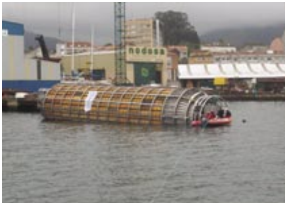
Aluminium shuttle used to remove the remaining cargo of fuel oil from the wrecks of the Prestige
