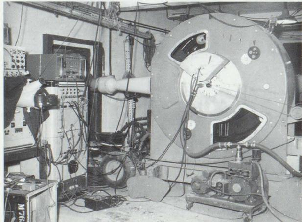
The C4 rotating mirror camera, also known as the 200-kilocycle camera, set up for use in a laboratory experiment
