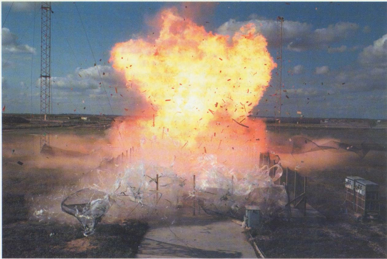
A recent high explosive trial at Foulness. High-speed rotating prism cameras, capable of recording at 10,000 fps, are used to measure the velocity of shock waves produced by the blast
