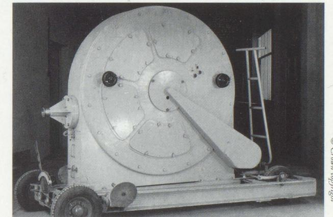
The Kerr Cell Cine camera, developed by AWE, could deliver exposure times as short as 0.1 of a microsecond at framing rates equivalent to 500,000 pictures per second
