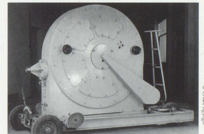
The Kerr Cell Cine camera, developed by AWE, could deliver exposure times as short as 0.1 of a microsecond at framing rates equivalent to 500,000 pictures per second
