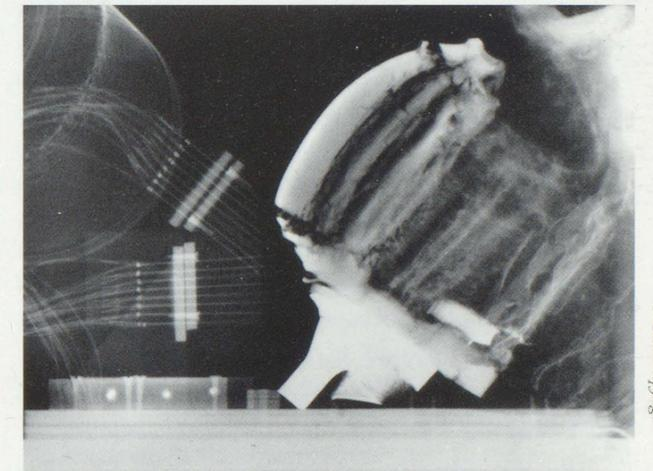
A nanosecond flash x-ray image of a high explosive trial, showing measuring probes and a flash bomb (used to provide illumination for optical rerecording) to the left
