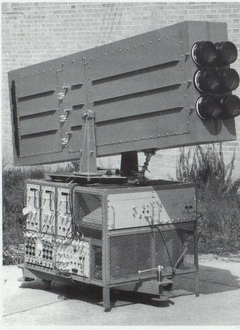
A six-channel Kerr Cell camera, with a focal length of 28 ft, which was used to photograph nuclear explosions at distances of several miles. Each channel could take a single photograph with an exposure time of about 0.1 of a microsecond (one tenth of a millionth of a second)
