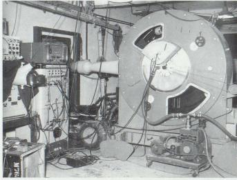
The C4 rotating mirror camera, also known as the 200-kilocycle camera, set up for use in a laboratory experiment
