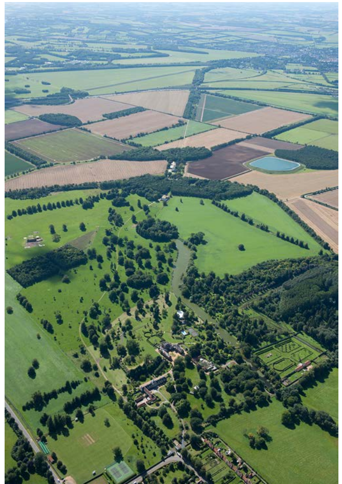
Figure 64 High oblique imagery that is unlikely to process well.
