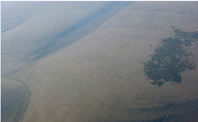
Figure 67 Haze in aerial imagery taken from a manned aircraft.
