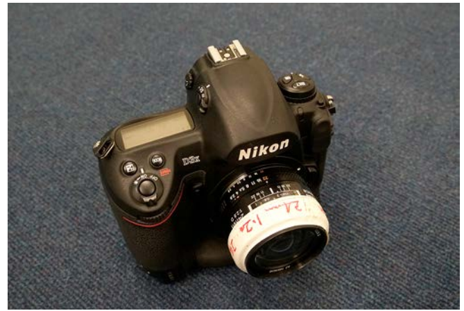
Figure 19 Prime lens taped to focus at 1.2m.
