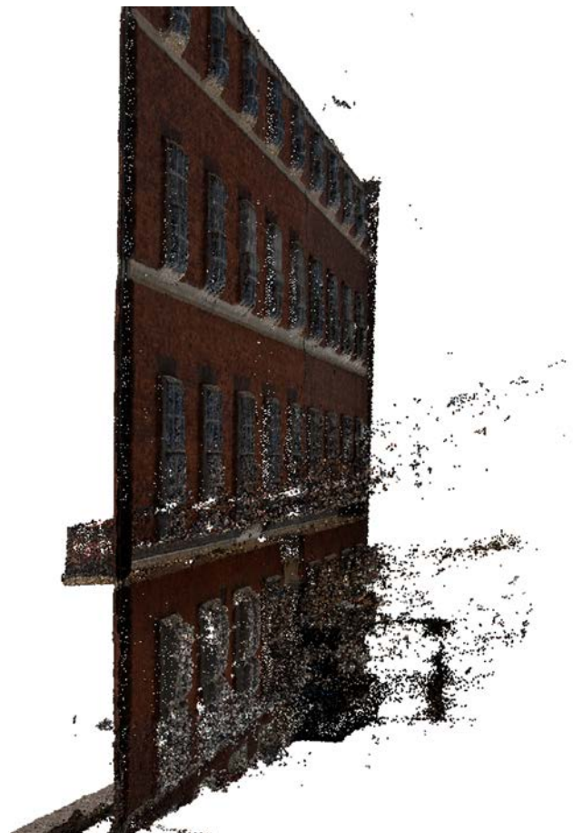
Figure 77 Extraneous geometry produced when photographing windows.
