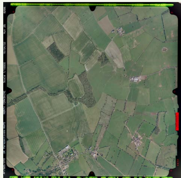
Figure 73 Aerial image with fiducial marks and other metadata.
