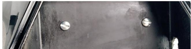
Once the holes have been cleaned and cleared of any swarf you can insert the 2 slotted Dzus fastener bolts through the holes, using the two black plastic washers on the under side of the tray to help hold the Dzus screw in place.
