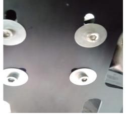
Put Loctite on the four bolts and line up all the bolts and holes, the design allows you to line up and adjust the plate before the final torque down of all the bolts.
