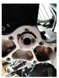
Clean the underside of the Triple tree you my need to clean out the threads I found my rear two were totally gunked up. A small stiff brush or even a tap will clear the threads
