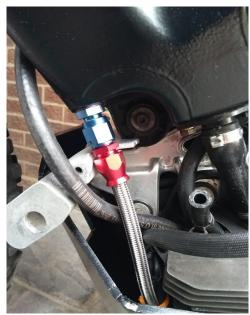
Unscrew the AN –Oil Tank adapter use the copper washer secure it into the oil tank.
