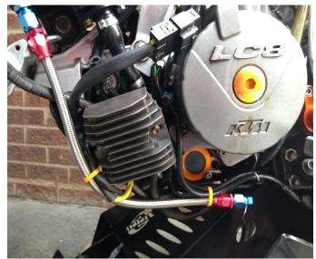
To drain the oil you simply have to undo the end cap using a 16mm socket. I found it easier to use another spanner to hold and secure the hose end fitting. On refitting I would recommend using a PTFE tape
