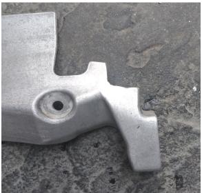
You will need to drain your oil and remove the top Battery plate, to cut out approximately a 1.5cm x 3cm.section This is to allow the line to run straight down with out putting pressure on the line and forcing a bend.
