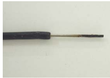
Carbon deposit which can prevent the electrode from working with Vet * Star
