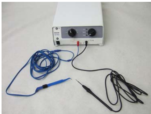
Note the insulator on the unused bipolar plug
