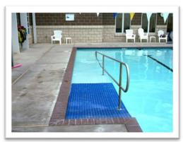
**Ramps** require more pool length than stairs but offer the advantage of "zero depth" and aquatic wheelchair entry.
