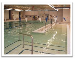
Stretch pools with bulkheads can also be considered – but many times a totally separate pool that has more Temperature Access and Depth control can be built for the cost of the bulkhead to create the "stretch" pool.
