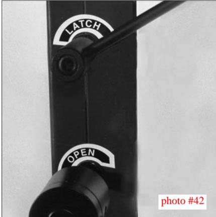
1. Install Latch Handle with adequate clearance for movement and tighten 1/8” set screw.
