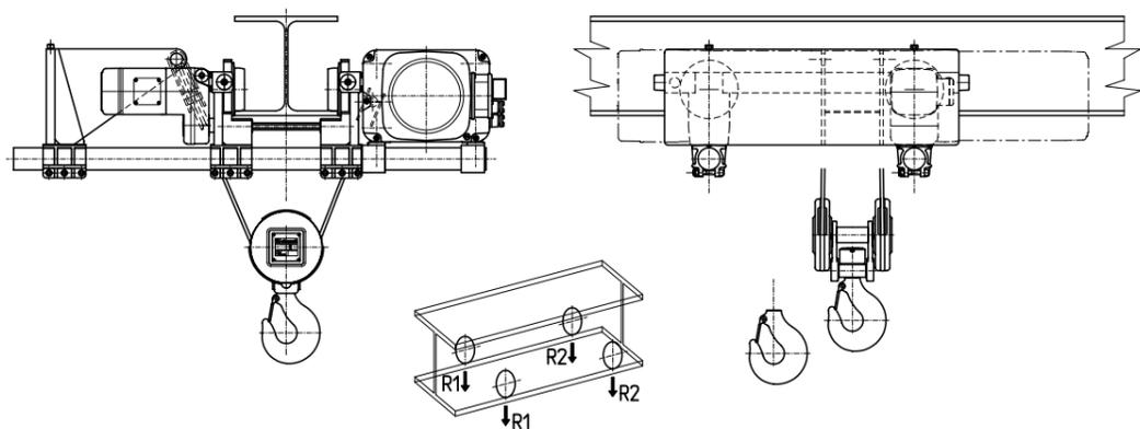
CHARIOTS BIPOUTRE DRT POUR PALANS ELECTRIQUES A CABLE DRH POSÉES OU SUSPENDUS
