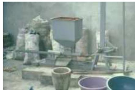
**Manual briquetting press for biomass waste residues in The Gambia**
