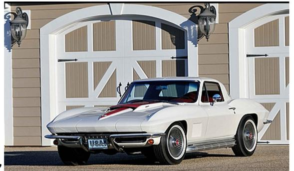
with the L36 427/390 HP engine, M20 4-speed manual transmission and 3.36 Positraction rear end; tinted glass, telescopic steering wheel, AM/FM radio, side exhaust and bolt-on aluminum wheels. Don's innate patriotism influenced his choice of colors: Ermine White paint, Red Stinger stripe and Red interior – a matchup he completed by replacing the factory Black wall rubber with a set of double White-and-Blue stripe tires.
