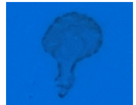
Figure 1 Stain on Paint Protection Film from a Leaf on uncoated C8 Corvette.
