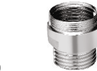
SPR-0724 | Nozzle For Shower Tube Top Thread - 24x1 Male for Perlmix Bottom Thread - 1/2" Male for Shower Tube
