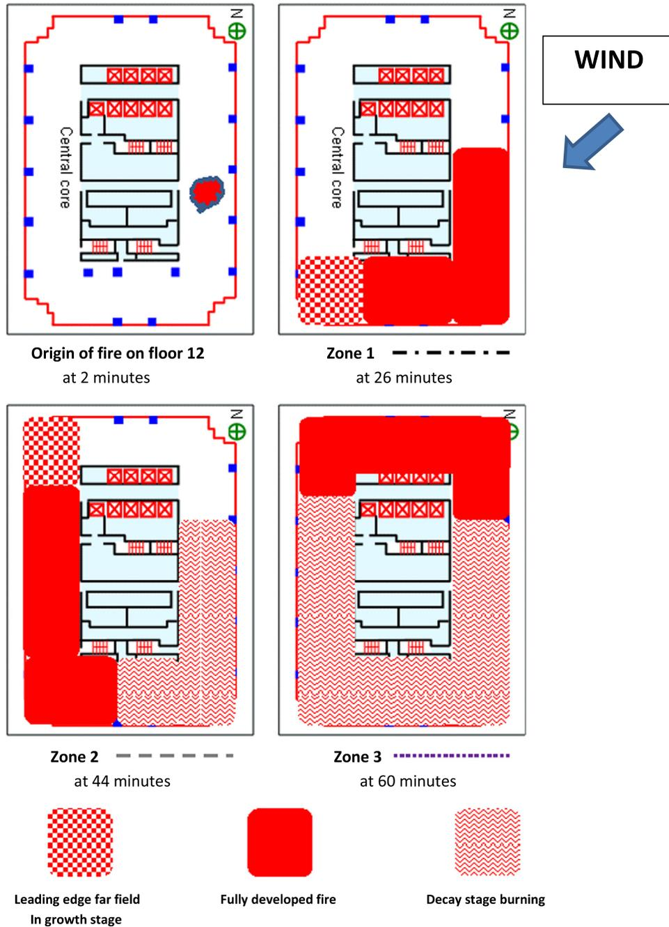
**Fig. 5.** Three-zone model for uncontrolled travelling fire spread (clockwise) at the Interstate Bank fire 1988; Adapted from an original at the *University of Manchester (school of Structural Fire Engineering) online 'one stop shop'* [13].
