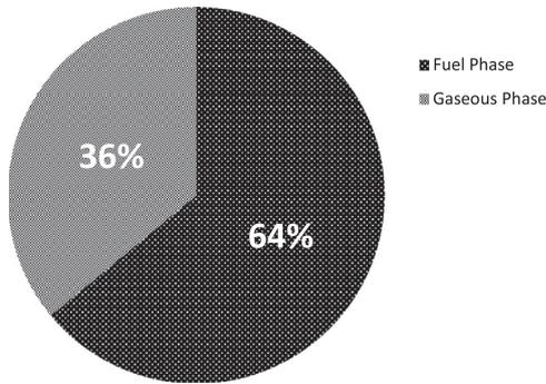
Fig. 10. The cooling ratio of applied firefighting water determined by full-scale ventilation controlled fire tests at Karlsruhe University (Fire Research Station) Tests in Germany 1984.
