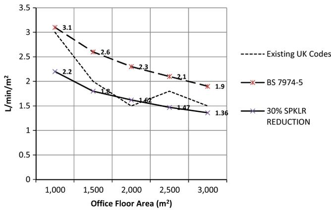
**Fig. 1.** A comparison of flow-rate density provisions across occupied floor space, between prescriptive UK regulations and the performance based BS PD 7974:5:2014 (excluding core areas) where a 30% sprinkler reduction has been applied.
