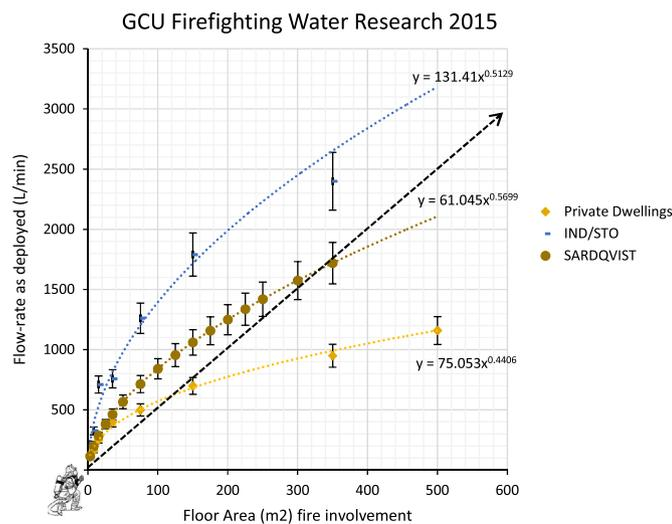
**Fig. 13.** The GCU research into firefighting water flow-rates used by UK firefighters at 5401 building fires with the  $A_{fire} \times 5$  fire-ground formula overlaid.
