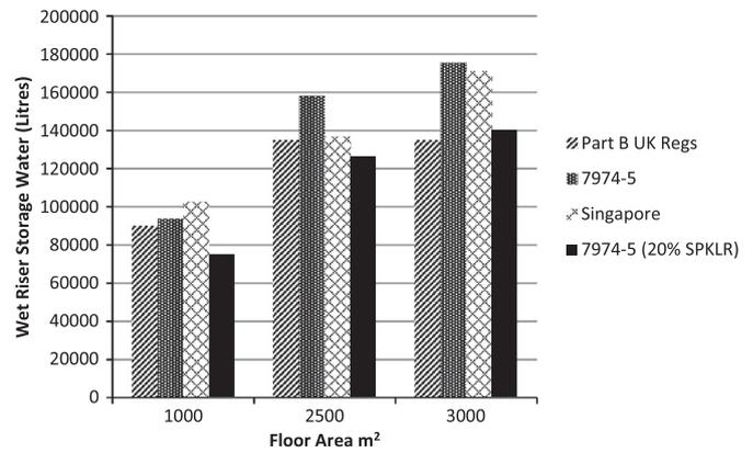
**Fig. 2.** The required or proposed water storage for wet rising fire main installations serving offices, providing 30 min continuous firefighting provision. An additional requirement for fire service connections to enable pumpers to augment the supply and maintain the flow-rate is also generally applied.
