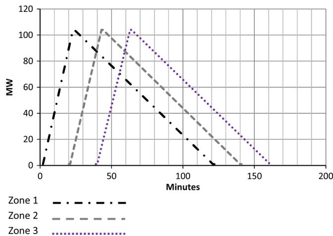
Fig. 6. Three zone model of heat release rates on the 12th floor at the First Interstate Bank 1988.
