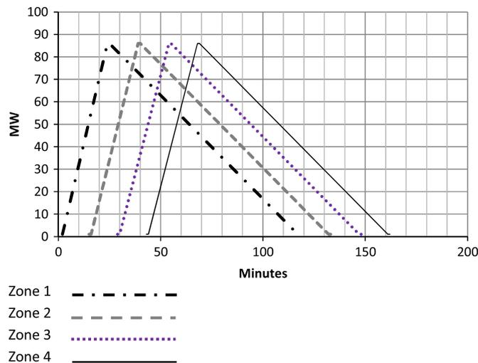
Fig. 7. Four-zone model of heat-release rates on the 12th floor at the First Interstate Bank fire 1988.
