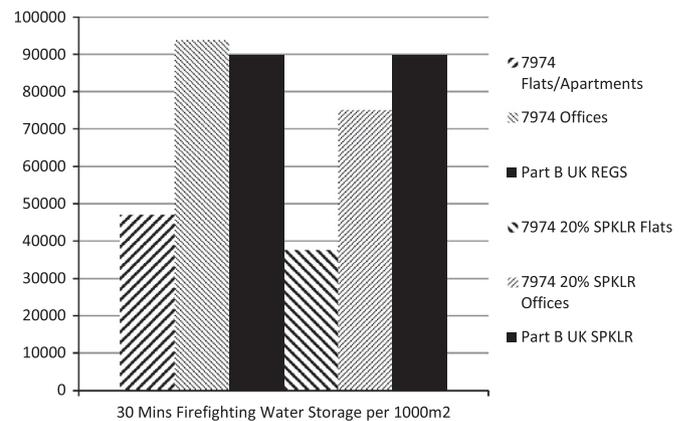
**Fig. 3.** A comparison (from left to right) of water storage requirements for a 30 min supply, between flats and offices using the BS PD 7974-5 methodology as opposed to the ADB approach where firefighting water provisions are the same for all building occupancies (providing maximum 45 m hose-run distances are achieved).
