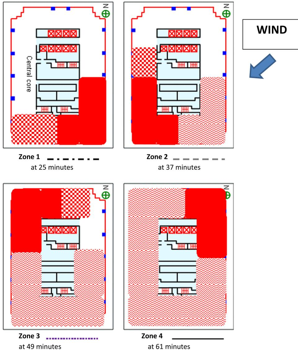
**Fig. 8.** Four-zone model for uncontrolled travelling fire spread (clockwise) at the Interstate Bank fire 1988; Adapted from an original at University of Manchester (school of Structural Fire Engineering) online ‘one stop shop’ [13].
