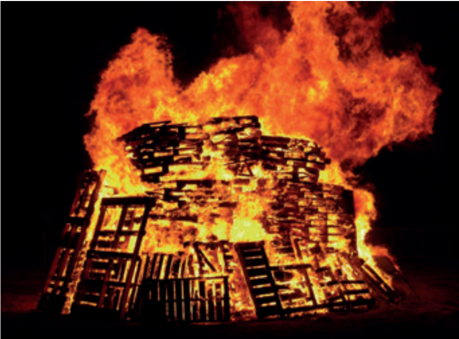
Figure 12.1: Burning pallets in the open – a fuel-controlled fire Photo courtesy of Terry Johnson
