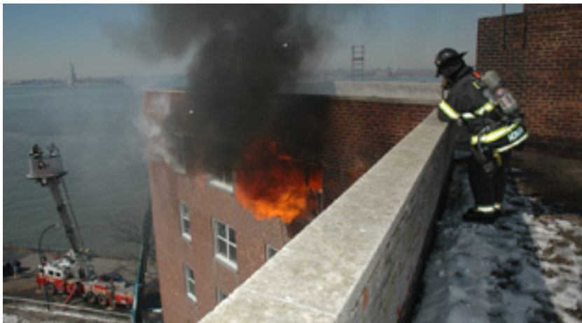
Figure 16.1: The Governors Island wind-driven fire tests undertaken by the National Institute of Standards and Technology (NIST), Fire Department New York (FDNY) and New York University 2008 Image courtesy of the National Institute of Standards and Technology (NIST) USA
