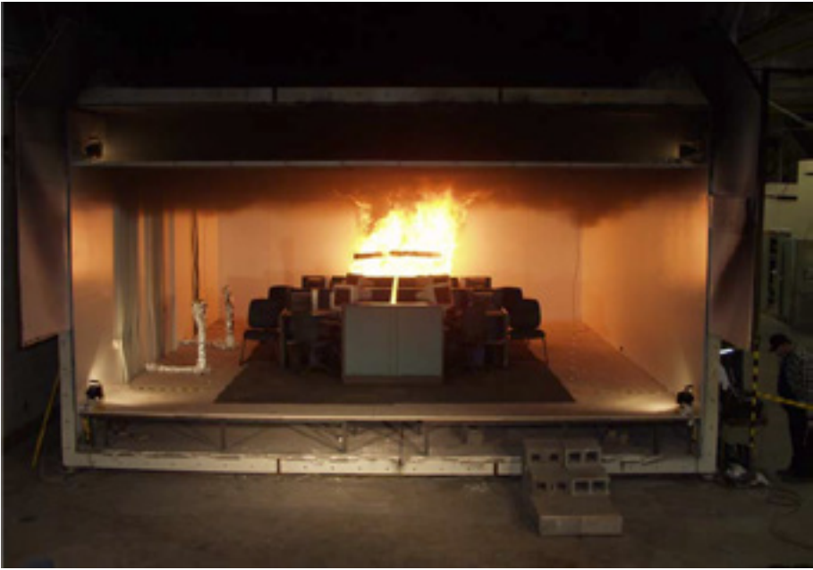
Figure 6.2: Multiple workstation enclosure fire experiment at CCAB at 20 secs into the fire growth. Image courtesy of National Institute of Standards and Technology (NIST)
