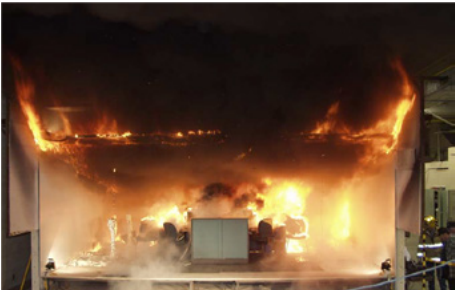
Figure 6.3: Multiple workstation enclosure fire experiment at CCAB at 300 secs demonstrating a heat release rate of 16 MW with four workstations fully involved just five minutes into the fire growth. Image courtesy of National Institute of Standards and Technology (NIST)
