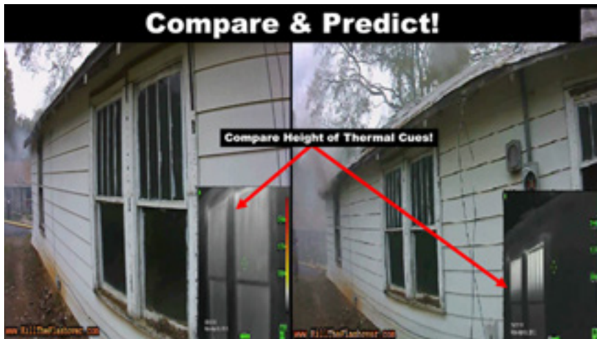
Figure 17.4: Thermal cues provided by a thermal imager from outside the building – such as the height of the heat layer and possibly the neutral plane Photos courtesy Project Kill the Flashover
