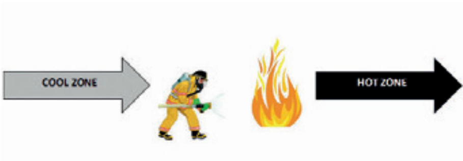
Figure 18.2: Flow-path cool zone between the inlet and the fire and hot zone between the fire and the outlet
