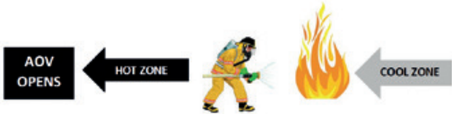
Figure 16.3: Exterior wind driven flow-path with AOV opened
