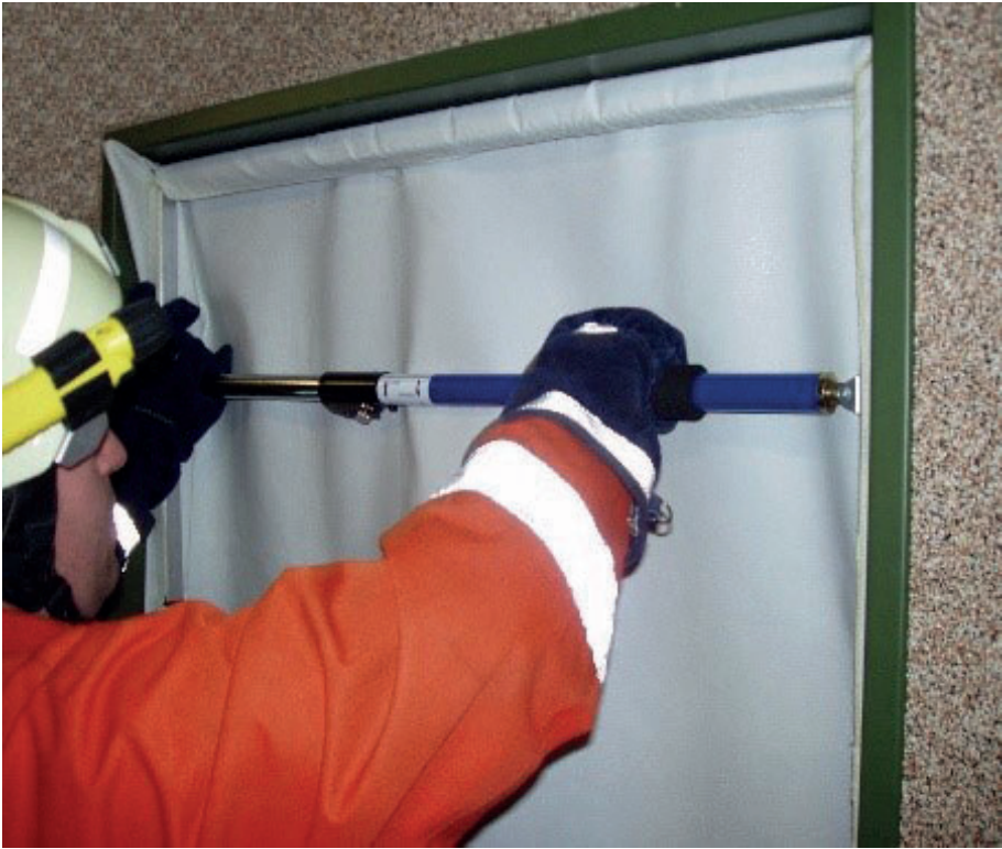
Figures 5.1: The smoke blocker is a tool for controlling smoke emissions from the fire compartment or main entry door in an apartment block. It serves to protect the corridor and stairs from smoke during firefighting intervention taking place. Images courtesy of Dr. Michael Reick http://www.rauchverschluss.de/index_e.htm
