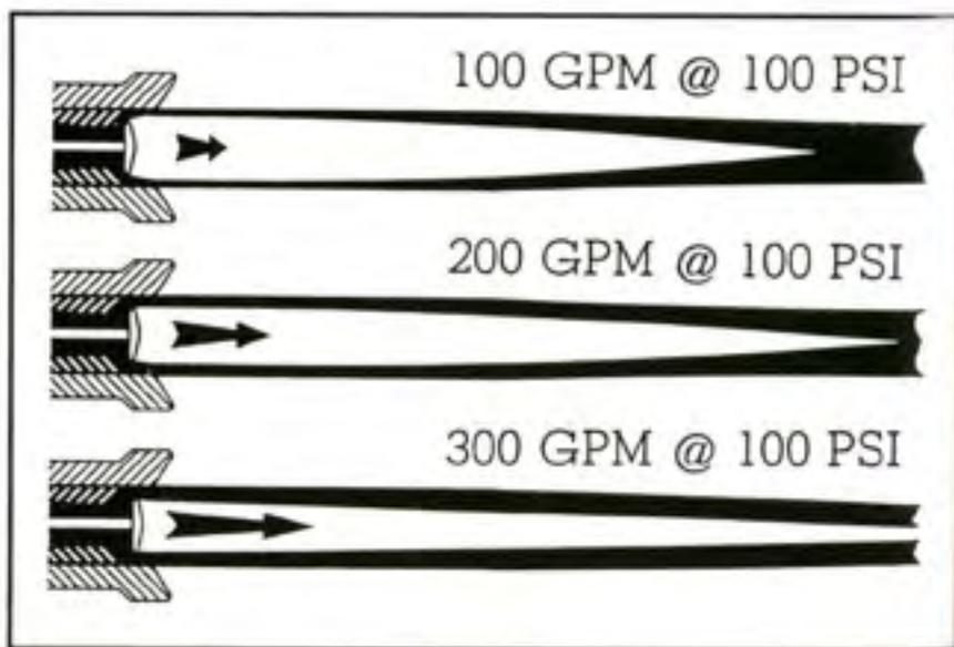
Figure 8-6 – Automatic nozzle – primary baffle varies the discharge at a constant nozzle pressure.
