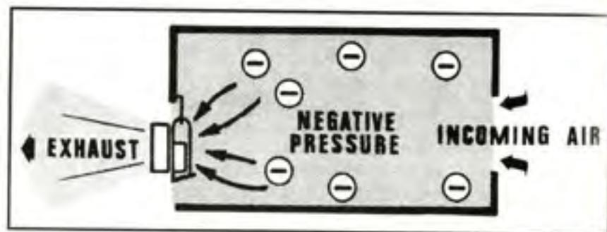
Figure 5:1 – A fan is used to initiate negative pressure ventilation.
