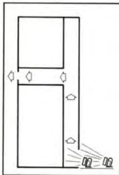
Figure 5:15 – Cross ventilation of a high-rise by in-line blowers.
