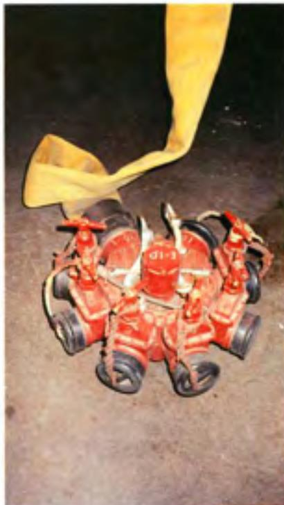
Above – A pressure relief valve fitted to a Boston pumper's intake to protect the pump where long lays of LDH are in use. Right – A 'Hanson Manifold' – as used by Seattle firefighters to lay a portable hydrant system. Below – A 10,000 l water 'pod' unit, as used by firefighters in Stockholm. The unit is able to shuttle the portable tanks (as seen) between the water source and the fire – all photos refer to Chapter 2.
