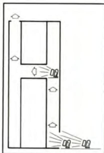
Figure 5:16 – Additional fans sited at upper levels to boost air-flow.
