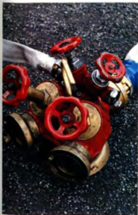
*Above – These Australian (CFA) firefighters advance on a fire behind the protection of a waterwall (Photo by Peter Baker, CFA Australia). Left – A Swedish hose divider, fed by a single 76 mm line, enables up to two 38 mm lines, and two 63 mm lines to be run from the outlets for attack purposes – Chapter 8.*
