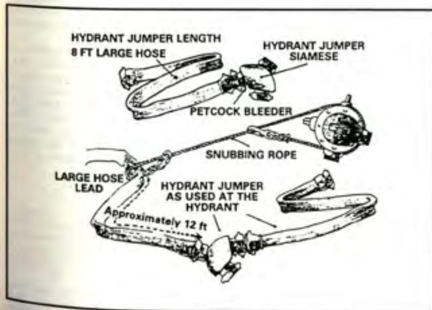
Figure 2:10 - SFFD hydrant jumper.
