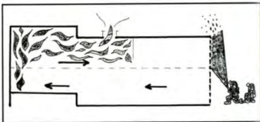
Figure 6:6 – A 'neutral plane' can be seen about one metre from the floor. Below this level the flow of air (and smoke) is towards the fire, while above it the flow is reversed. Before firefighters open the door to a free compartment they should inert the air outside it with a burst of fog. (Note: only the finely divided particles of a water fog are able to suspend in air – the droplets from a 'spray' nozzle may be too heavy to create this effect.)
