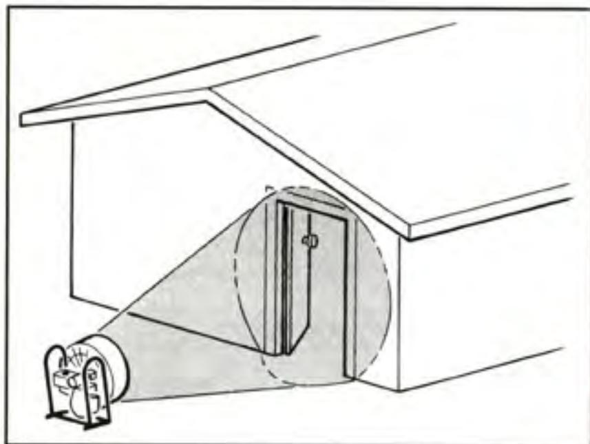
Figure 5:4 – On its own, a single blower should be positioned so the cone of pressurised air just covers the entrance opening.
