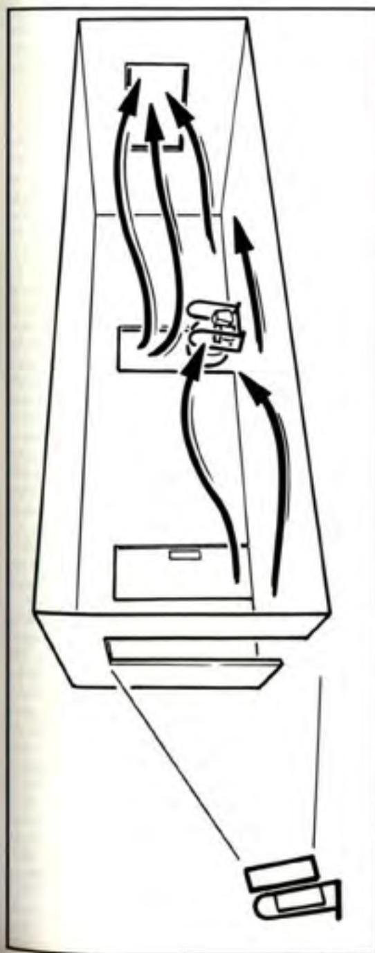
Figure 5:11 – Using PPV fans to ventilate enclosed areas with no openings.
