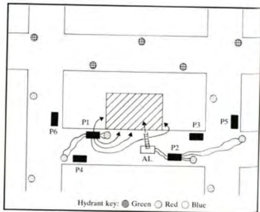
Figure 2:15 - Ineffective use of hydrant grid.
