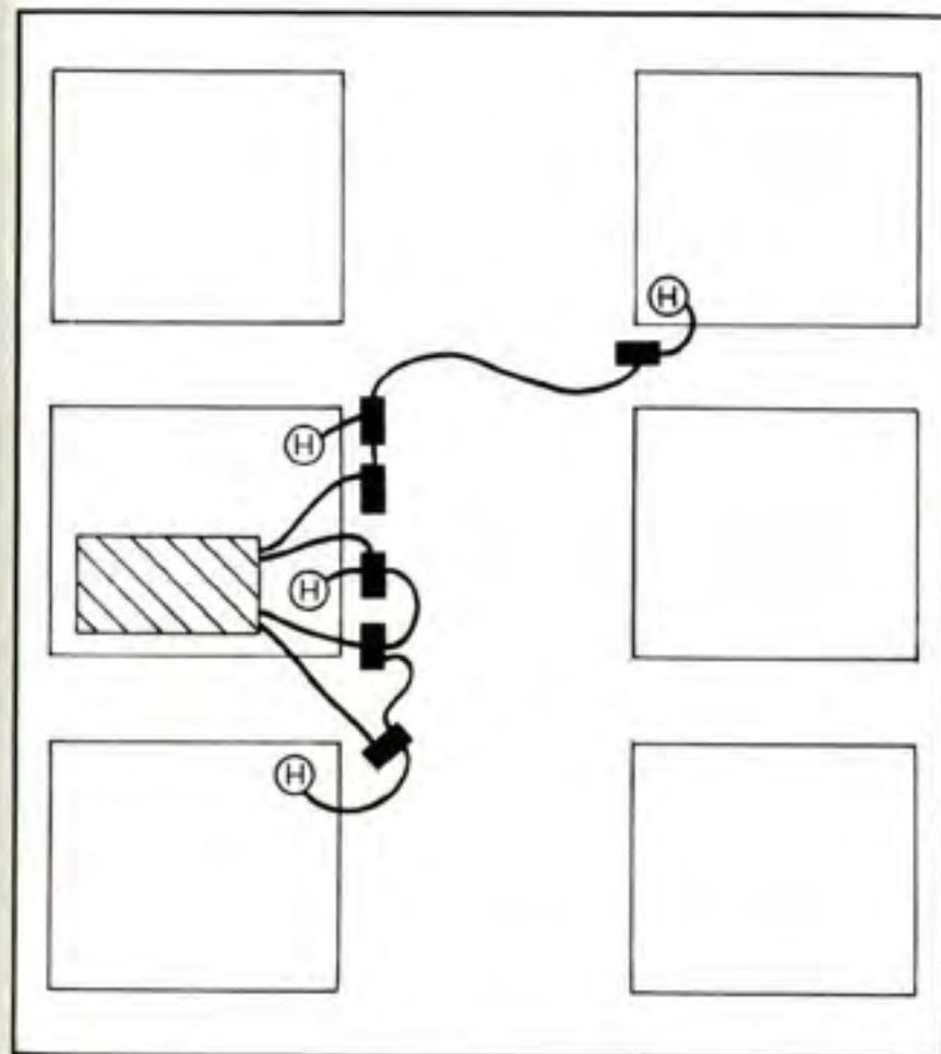
Figure 9:1 – Note the supply hose layout at the interstate Bank fire – Los Angeles. The pumps are sited directly on the hydrants to 'boost' the pressure, before feeding the supply into additional pumps charging the standpipes. (Fire building shaded).
