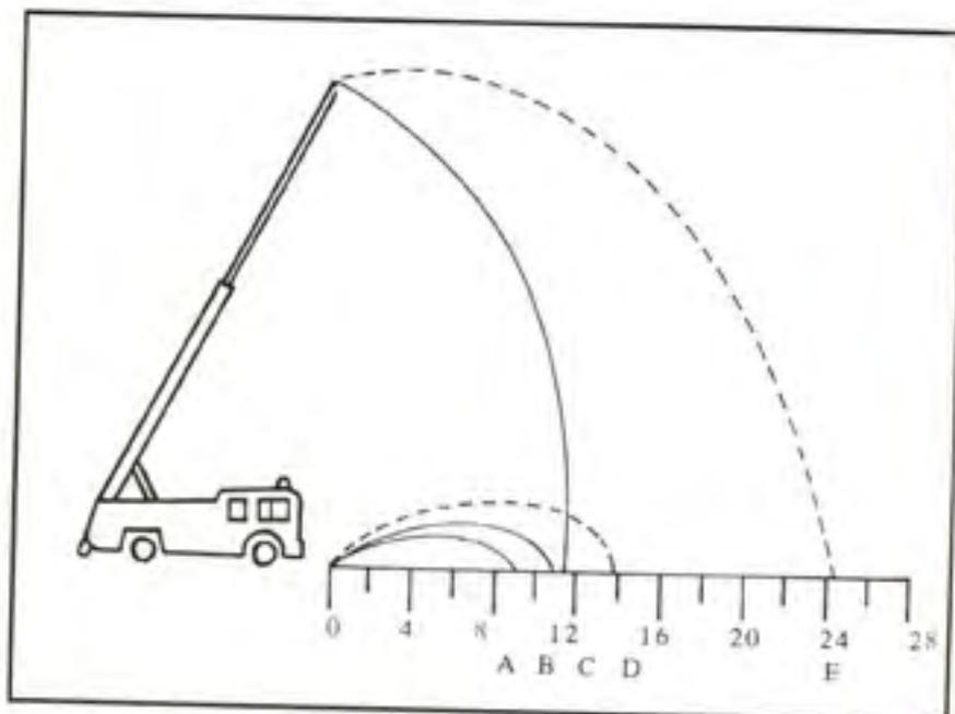
Figure 2:17 - The effect of fire stream power.
