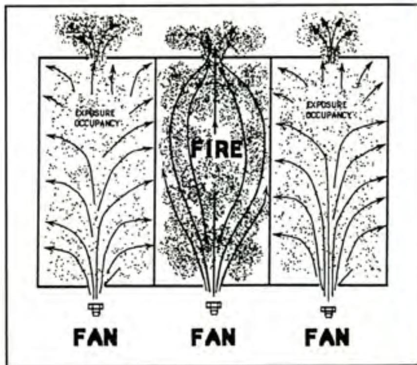
Figure 5:18 – The use of PPV fans to confine a fire.
