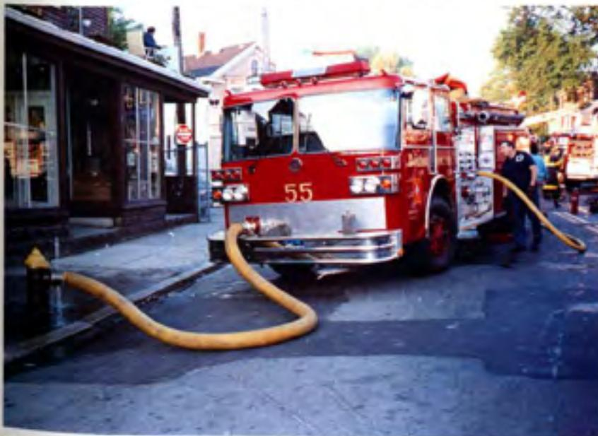
A Boston fire pumper sites directly on the hydrant to boost the supply. A line of 125 mm hose is also used to reduce frictional loss and maintain a high residual pressure at the pump, enabling the full flow (LPM) to be drawn from the hydrant – see Chapter 2.
