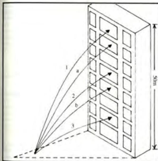
Figure 8:3 – Effect of hydrant grid classification on stream reaches.
