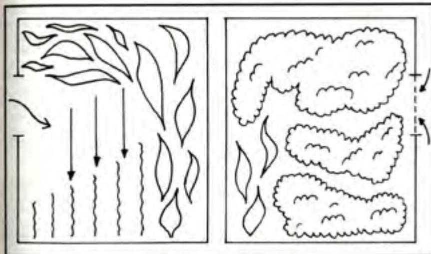
Figure 6.2 – Radiation induced (left) and ventilation induced (right).
