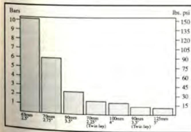
Figure 2.2 – Frictional loss in hoselines 100 m (333 ft) in length flowing 1,500 LPM (400 GPM US).
