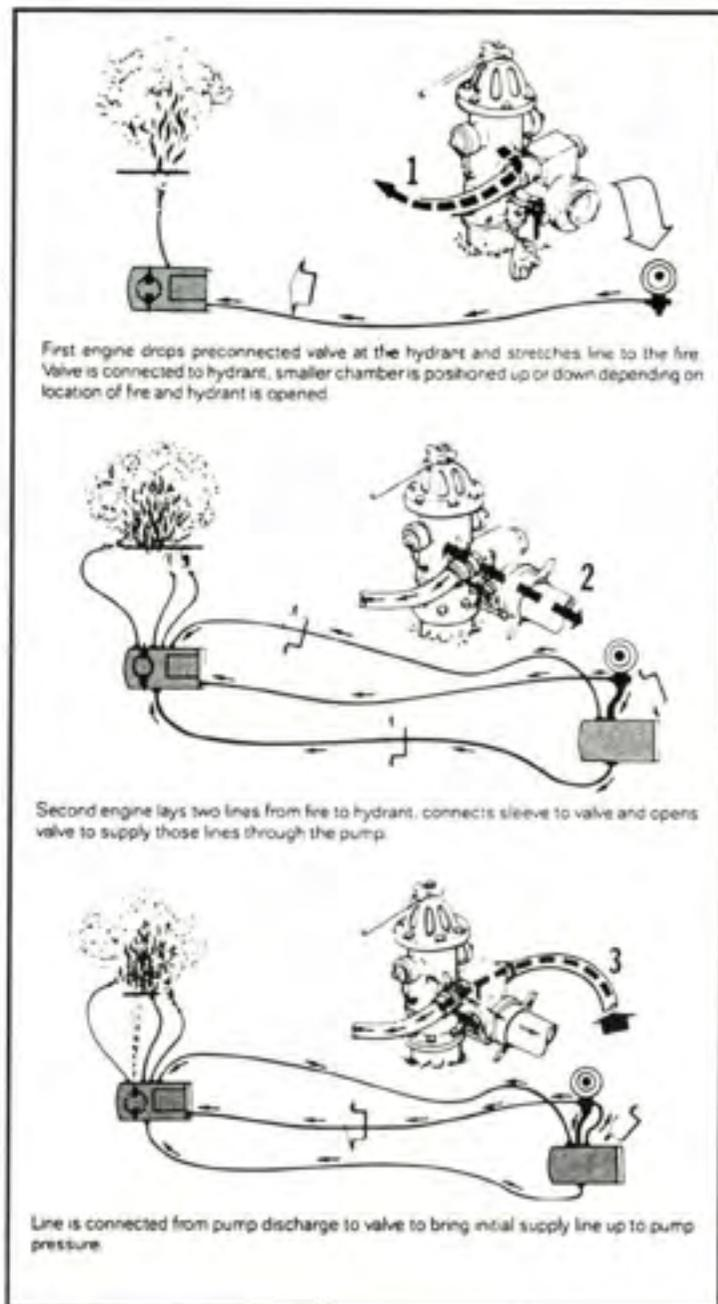
Figure 2:9 - Hydrant assist valve.
