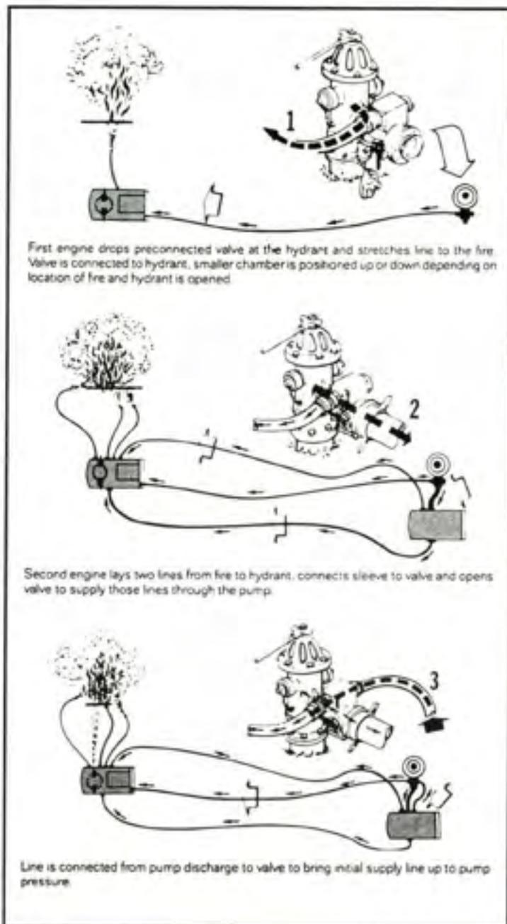
Figure 2:9 - Hydrant assist valve.
