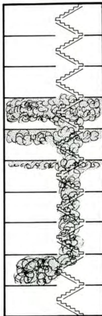
Figure 5:14 – The 'stratification' effect of smoke in tall buildings.
