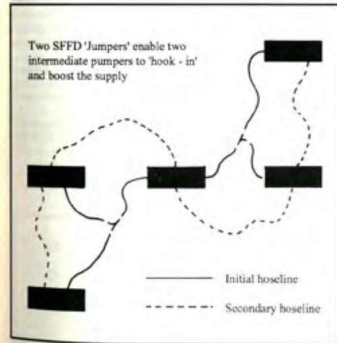
Figure 2:14 SFFD water relay utilising 'jumpers' in line.
