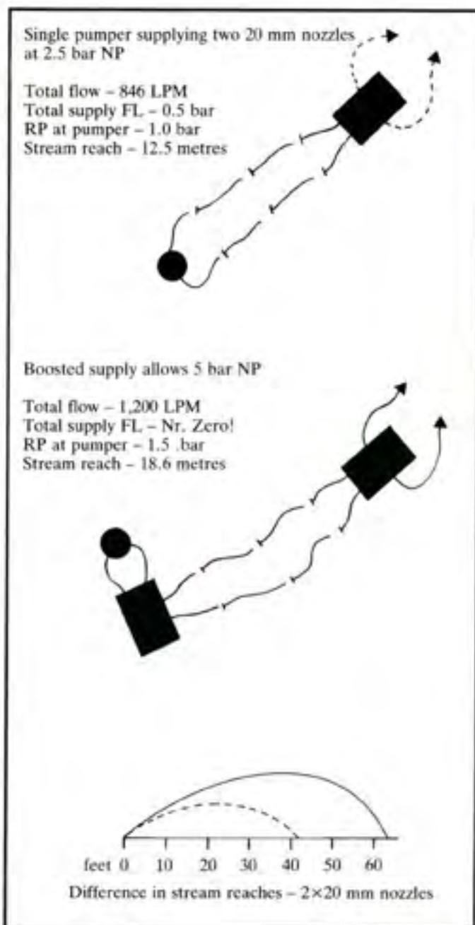
Figure 2:8 - Effect of booster pump
