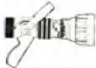
H1VPG (Previously H1FT-VPG) Fully automatic nozzle with a flow capacity of 50-350 GPM. Includes pressure assisted flush without shutting down, patented slide valve for turbulence free nozzleman flow control, six detent flow positions, molded rubber teeth for full fit "power fog" and "Gasket Grabber" inlet screen. Integral rubber coated pistol grip is mounted below the valve handle. All lightweight materials. Can be used with 2-1/2" line with HA adapter. Full time swivel is standard.
