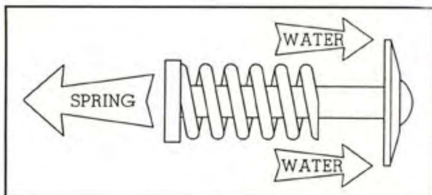
Figure 8-5 – Automatic nozzle – pressure control mechanism.
