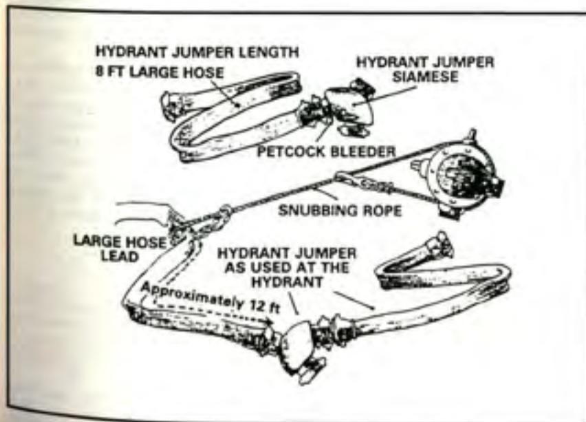
Figure 2:10 - SFFD hydrant jumper.
