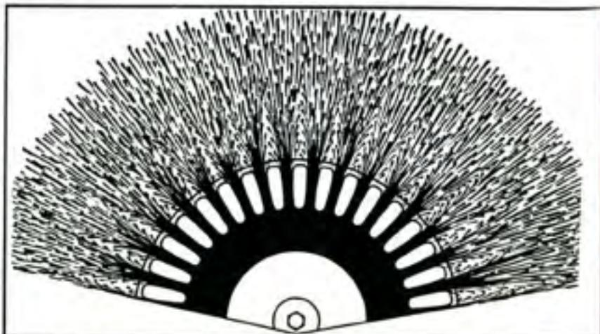
Figure 3:7 - Fog pattern-moulded rubber teeth provides full fill to the cone with no 'fingering'.
