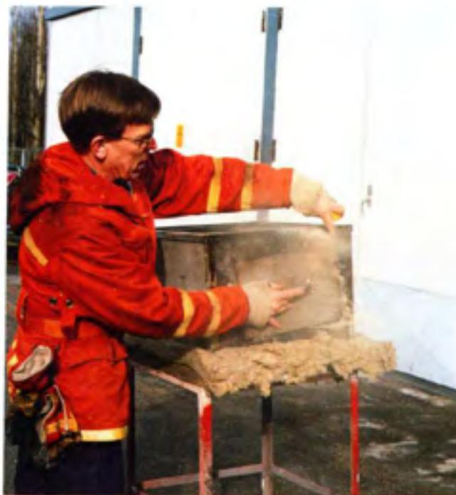
A scaled-down model of the container is used to teach firefighters some important aspects of fire behaviour, in relation to flashovers and backdrafts, prior to taking part in container training – Chapter 6.
