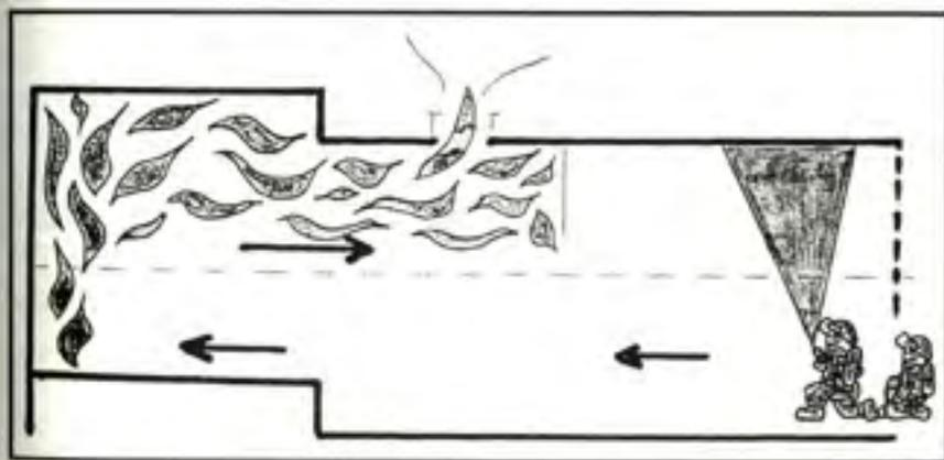
Figure 6:7 – On entering a fire compartment, firefighters apply the 'water test' by directing brief 'pulses' of fog immediately above their heads. This will determine the temperature in the fire gas layer above them. If it is cool, the water will fall back on them.
