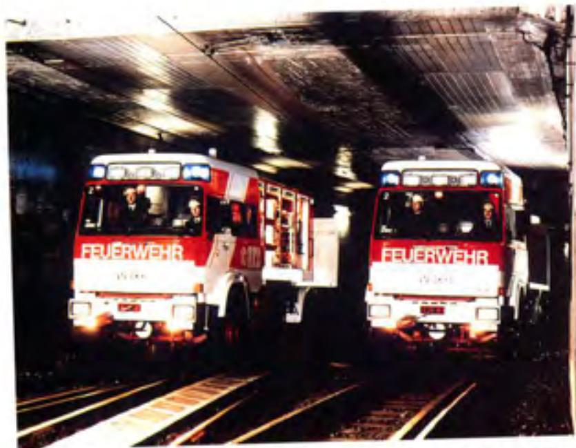
These fire trucks in Frankfurt are designed to run on either road wheels, or specially fitted track wheels – see Chapter 10. (Photo by Iveco Magirus).
