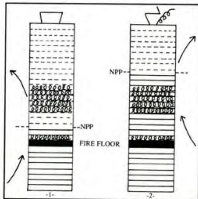
Figure 4-9 - Vertical ventilation in this case raises the NPP and creates unfavourable air flows on the upper levels.
