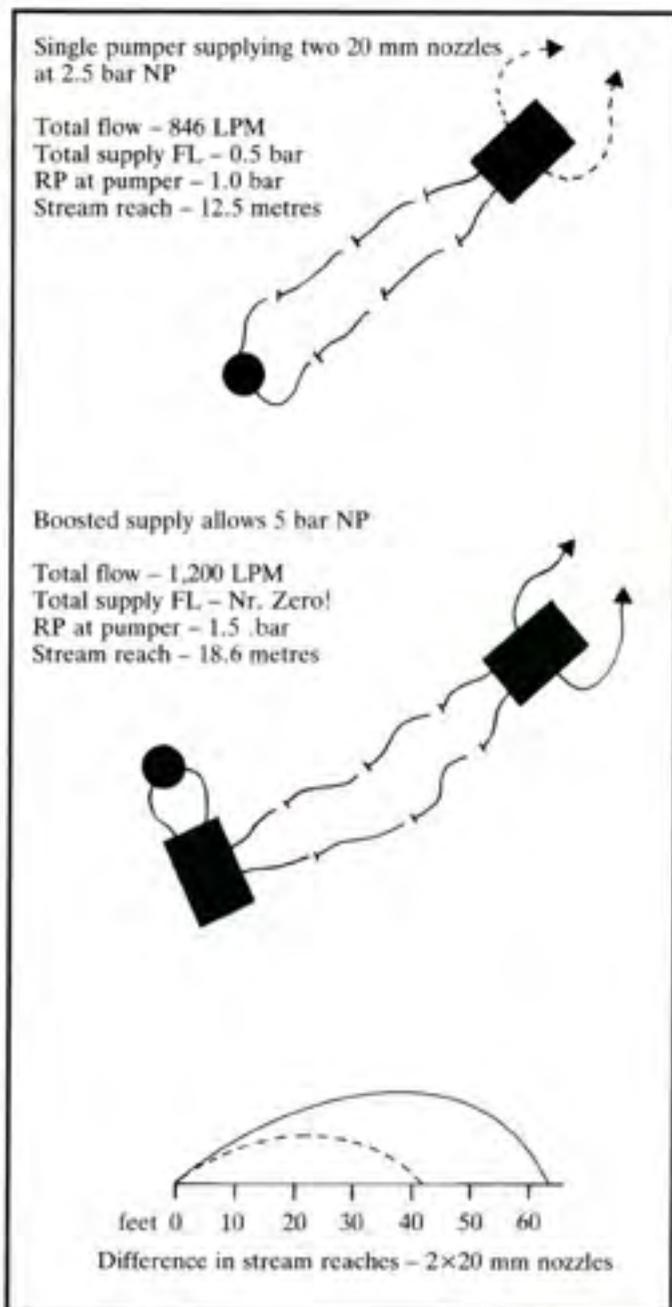
Figure 2:8 - Effect of booster pump
