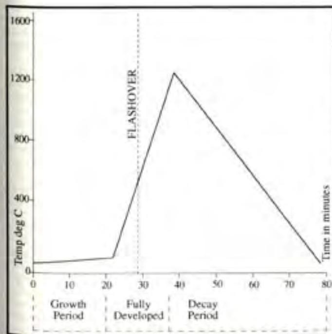
Figure 6.1 - The time/temperature fire profile: the curve represents the average temperature of a compartment fire determined under test conditions.
