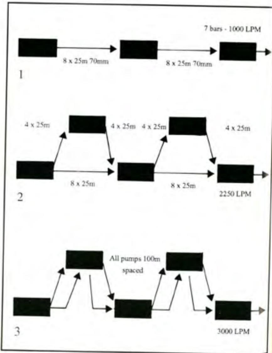
Figure 2:13 - Pump spacing for water-relay system.
