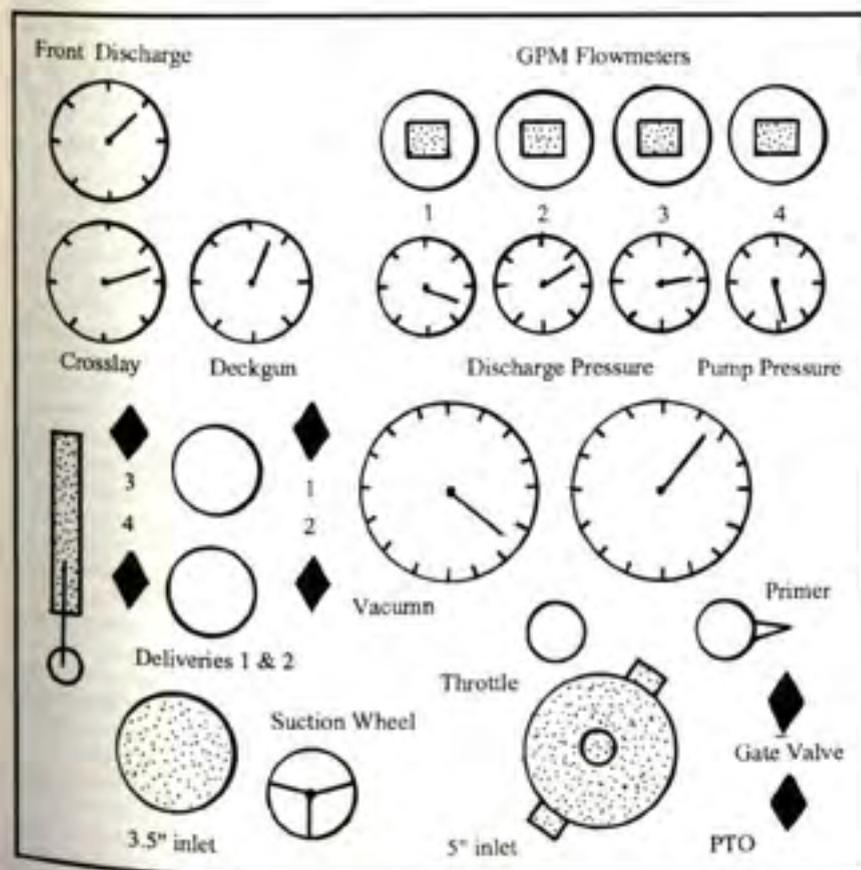
Figure 2:18 - New York firefighters have benefit of this pumper control panel.
