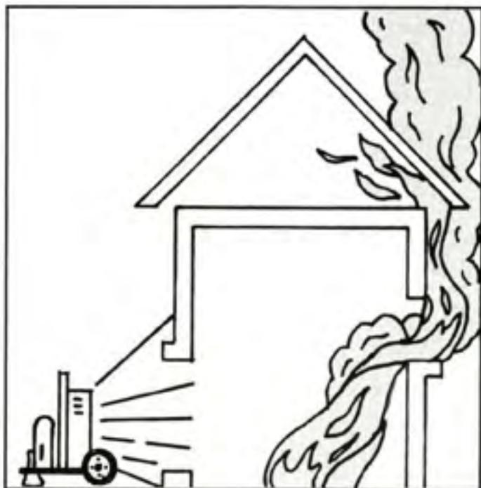
Figure 5:20 – Fire extension into the roof space has been a common problem where PPV is concerned and the situation should be anticipated and checked before the fire is allowed to escalate beyond control.
