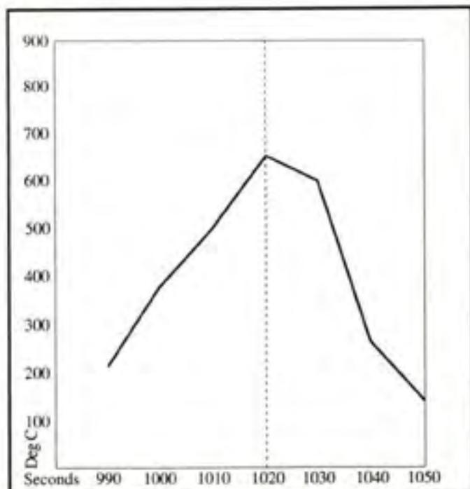
Figure 6:5 – Temperatures at 1.6 m from the floor during an extinguishing cycle in a fire simulator (extinguishing of the gas layer begins at 1,020 seconds).
