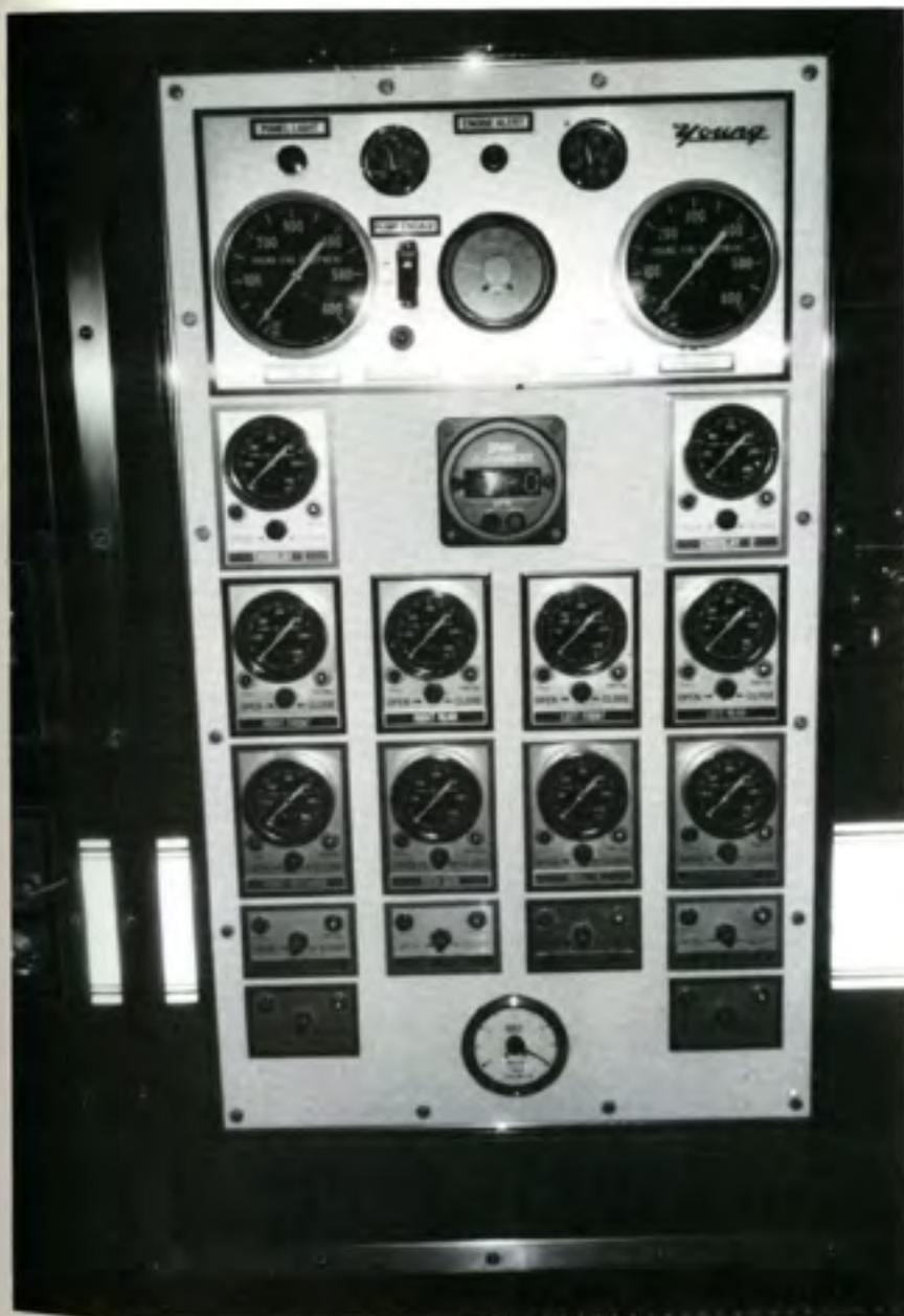
The 'Hi-tec' control panel fitted to the very latest line of fire pumpers in Miami (6,000 LPM). There is a flowmeter that registers total output (LPM) and each of the ten discharge ports, including the 'Deck-Gun', have their own pressure gauges. Output is initiated through finger-tip control knobs (as seen under each pressure gauge) – see Chapter 2.
