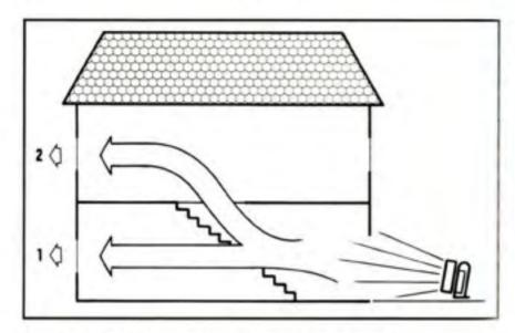
Figure 5:10 - The PPV concept utilised in a multi-storey structure.
