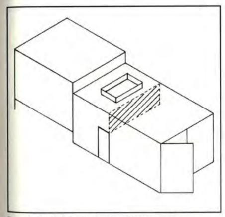
Figure 6:4 - Room fire simulator - manufactured container design.
