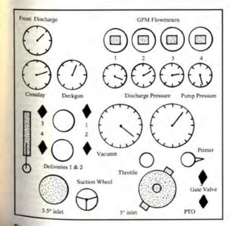
Figure 2:18 - New York firefighters have benefit of this pumper control panel.
