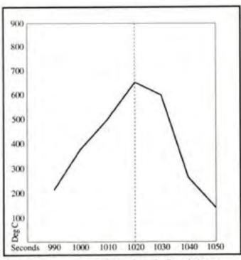
Figure 6:5 – Temperatures at 1.6 m from the floor during an extinguishing cycle in a fire simulator (extinguishing of the gas layer begins at 1,020 seconds).
