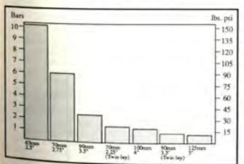
Figure 2:2 -Frictional loss in hoselines 100 m (333 ft) in length flowing 1,500 LPM (400 GPM US)
