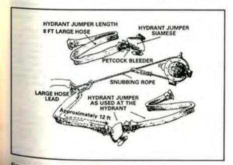
Figure 2:10 - SFFD hydrant jumper.
