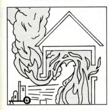
Figure 5:21 – An incorrect placement of the PPV fan is likely to cause a 'blow-back' at the point of entry. The fan above is sited too close to the opening and the cone of air is unable to cover the upper section.
