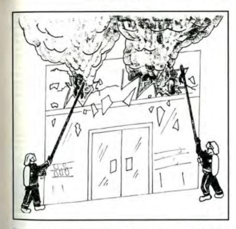
Figure 4:6 – Before ventilating a compartment it is important to ensure that the attack team is ready with a charged hoseline and the added protection of CABA – with masks in place. The correct method of venting a glass shop-front is shown above. A 'coverline' should be sited to the side of the opening.
