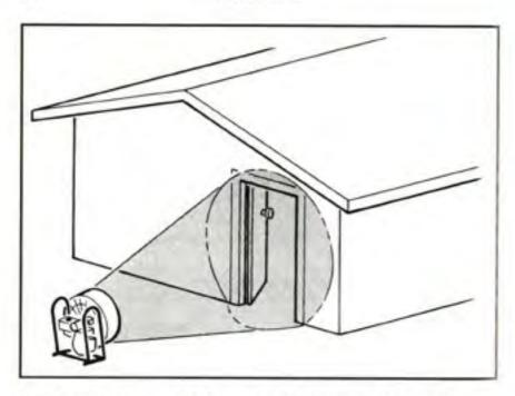
Figure 5:4 – On its own, a single blower should be positioned so the cone of pressurised air just covers the entrance opening.
