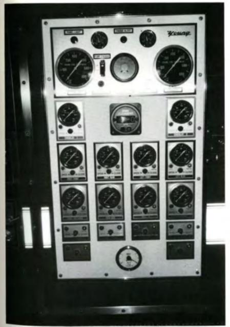
The 'Hi-tec' control panel fitted to the very latest line of fire pumpers in Miami (6,000 LPM). There is a flowmeter that registers total output (LPM) and each of the ten discharge ports, including the 'Deck-Gun', have their own pressure gauges. Output is initiated through finger-tip control knobs (as seen under each pressure gauge) – see Chapter 2.
