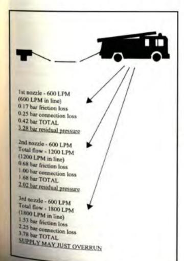
Figure 2:4 – Hoselay # 2 – single 100 mm.
