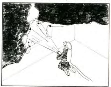
Figure 4:7 – With a nozzle position located a few feet from the window, and a fog cone of 55-60 degrees, the Venturi effect in the stream will assist in displacing the smoke from the compartment.
