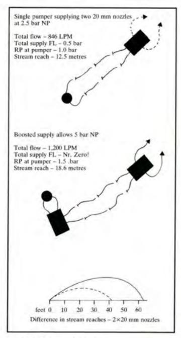
Figure 2:8 - Effect of booster pump
