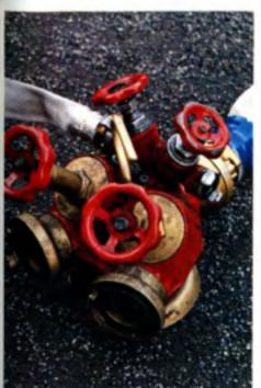
Above – These Australian (CFA) firelighters advance on a fire behind the protection of a waterwall (Photo by Peter Baker, CFA Australia). Left – A Swedish hose divider, fed by a single 76 mm line, enables up to two 38 mm lines, and two 63 mm lines to be run from the outlets for attack purposes – Chapter 8.
