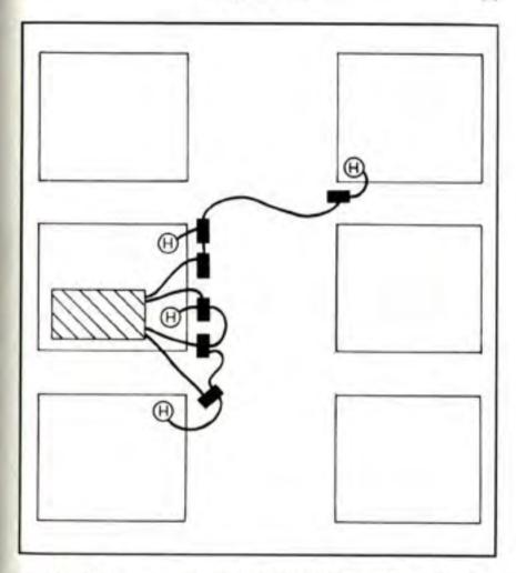
Figure 9:1 – Note the supply hose layout at the interstate Bank fire – Los Angeles. The pumpers are sited directly on the hydrants to "boost" the pressure, before feeding the supply into additional pumps charging the standpipes. (Fire building shaded).
