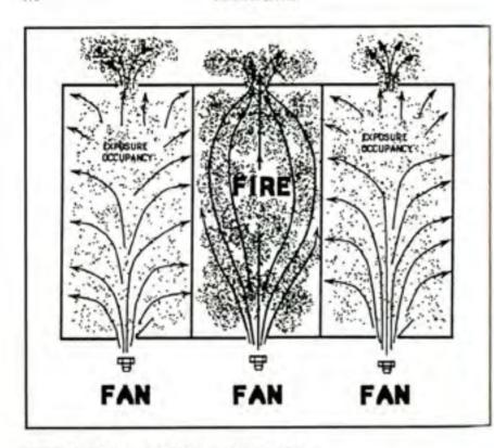
Figure 5:18 - The use of PPV fans to confine a fire.
