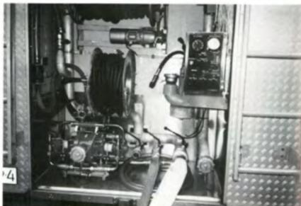
Top left – Although this Miami MPO is sited some distance from the fire, he is in direct contact with the firefighters on the nozzle. Top right – The 'basic' pumper control panel of an Amsterdam fire pumper (3,000 LPM). Above – The 'basic' pumper control of a Stockholm fire pumper (1,800 LPM) – all photos refer to Chapter 2.
