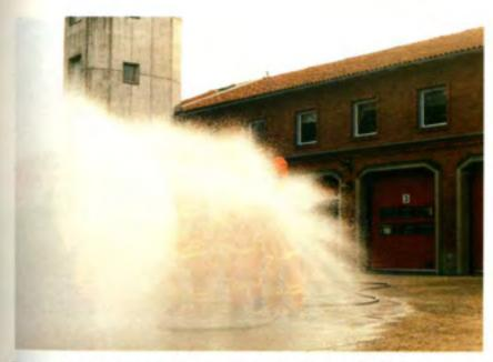
The effect of 'fingering' is clearly apparent in the fog stream on the right, when compared with the full fog pattern on the left – see Chapter 3.
