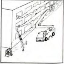
Figure 5:17 – US firefighters utilise a PPV fan to create a 'false wind' across the face of the building, enabling a better view for ladder placements and rescue operations.
