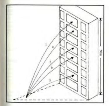
Figure 8:3 – Effect of hydrant grid classification on stream reaches.
