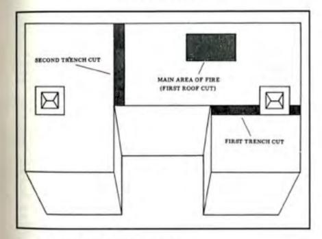
Figure 4:4 - Three types of roof ventilation cuts.
