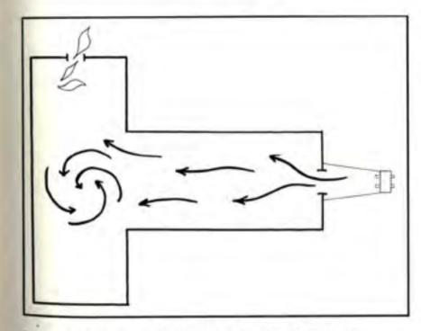
Figure 5:19 – The 'swirling' effect noted where PPV is used in 'T' shaped compartments.
