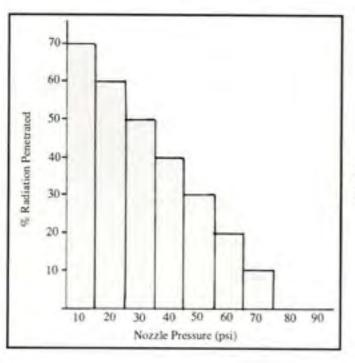
Figure 3:8 – Effect of radiant heat on the nozzle.
