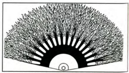
Figure 3:7 – Fog pattern-moulded rubber teeth provides full fill to the cone with no 'fingering'.
