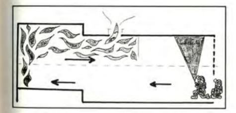
Figure 6:7 – On entering a fire compartment, firefighters apply the 'water test' by directing brief 'pulses' of fog immediately above their heads. This will determine the temperature in the fire gas layer above them. If it is cool, the water will fall back on them.
