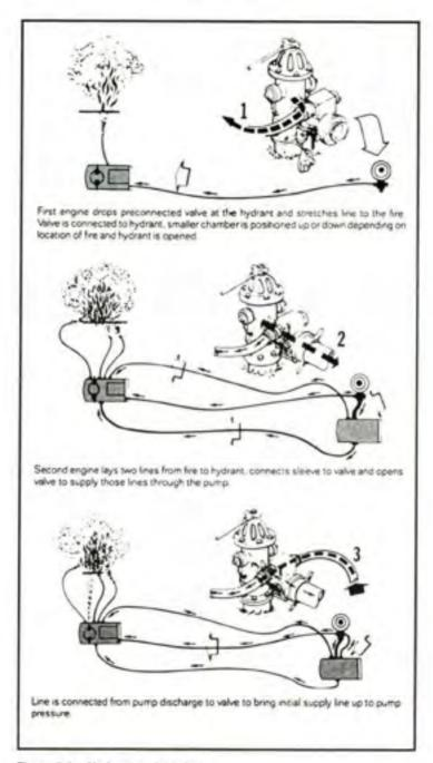
Figure 2:9 - Hydrant assist valve.
