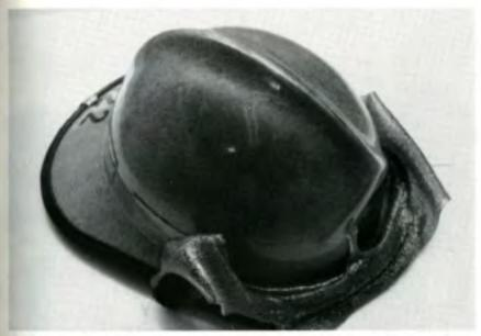
The severity of conditions encountered inside the Swedish flashover simulator places all items of protective equipment under great stress – Chapter 6.
