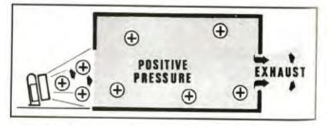
Figure 5:2 - The basic concept of positive pressure ventilation (PPV).
