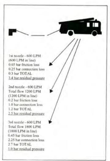
Figure 2:5 -Hoselay # 3 single 125 mm.
