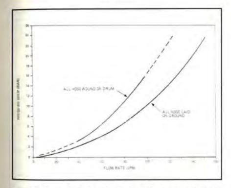
Figure 3:5 – Pressure losses versus flow for three 18.3 m lengths of 19 mm bore hosereel.
