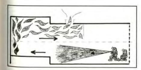
Figure 6:8 — Before firefighters advance into the compartment, full use is made of the air-flow below the neutral plane. A brief burst of fog is applied at low level into the compartment, enabling the water droplets to be drawn in towards the seat of the fire. While this is a good tactic in a real fire it should be avoided in a container simulation, where it should be the intention not to extinguish the fire's seat.
