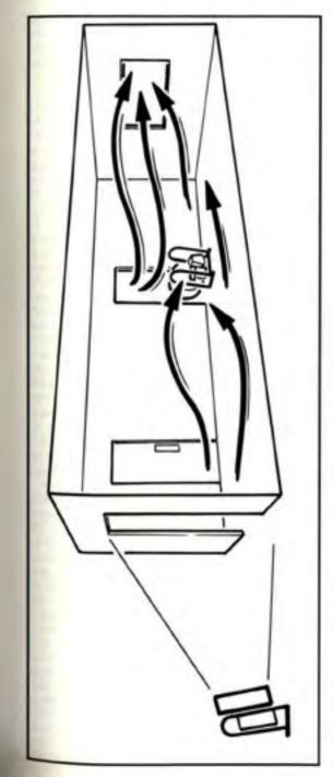
are 5:11 - Using PPV fans to ventilate enclosed areas with no openings.
