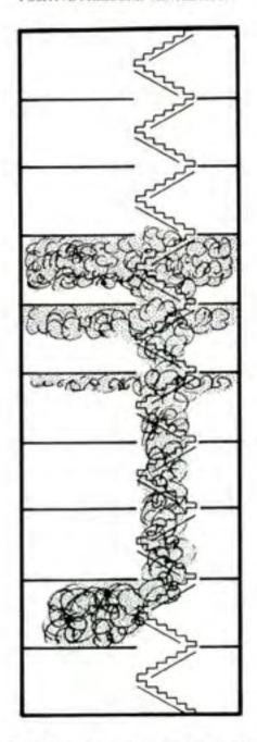
Figure 5:14 - The 'stratification' effect of smoke in tall buildings.
