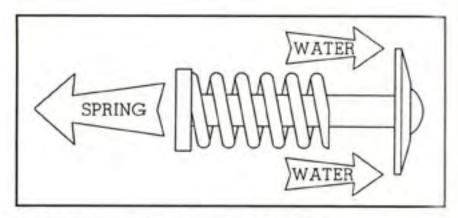
Figure 8:5 - Automatic nozzle - pressure control mechanism.
