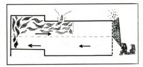
Figure 6:6 – A 'neutal plane' can be seen about one metre from the floor. Below this level the flow of air (and smoke) is towards the fire, while above it the flow is reversed. Before firefighters open the door to a free compartment they should inert the air outside it with a burst of fog. (Note: only the finely divided particles of a water fog are able to suspend in air – the droplets from a 'spray' nozzle may be to heavy to create this effect.)
