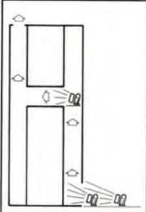
Figure 5:15 - Cross ventilation of a highrise by in-line blowers.
