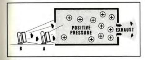
Figure 5:5 - Effective placement of twin PPV fans.
