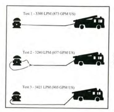
Figures 2:6 – Results of Starkville flow tests.
