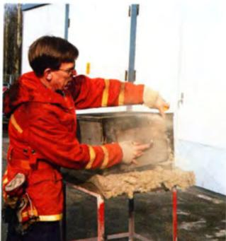
A scaled-down model of the container is used to teach firefighters some important aspects of fire behaviour, in relation to flashovers and backdrafts, prior to taking part in container training – Chapter 6.
