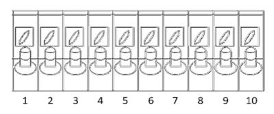
**(1,2) Batt Temp:** Battery Temperature Sensor has no polarity and is needed for voltage correction when using lead acid batteries.
