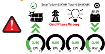
If the Sol-Ark screen shows **Grid Phase Wrong** there is a phasing issue with your wiring and it may cause overload faults (F18, F26, F34) <u>even</u> with the Load breaker **off** and **WILL CAUSE DAMAGE if left unchecked**.
