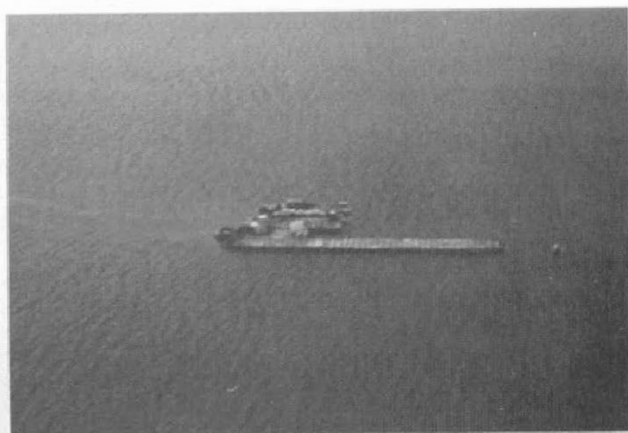
FIGURE 6-11. WARPING TUG CAUSEWAY FERRY.
