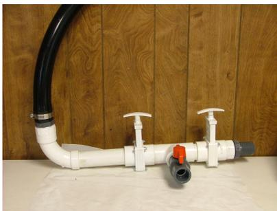
**Valve Assembly (Gate and Ball Valves)**
