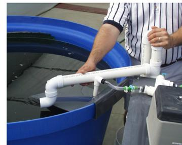
**Figure 10: Aim water outlet to encourage circular flow**
