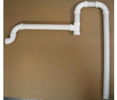
**Completed Airlift Water Pump Assembly**
