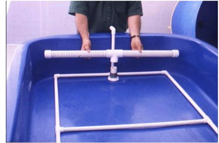
**Figure 8: The Air Ring and Inflow Header go into the Tray**
