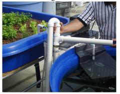
Figure 9: Push Return Flow and Skimmer pipes down onto top of Airlift pipe
