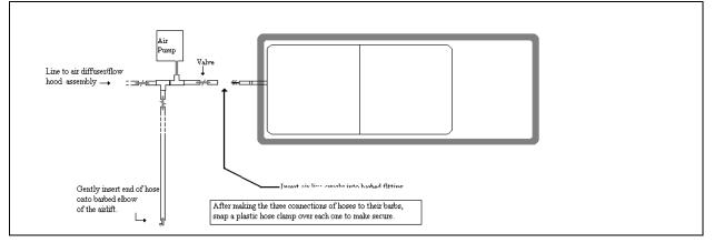
Figure 7: Layout of the air supply lines
