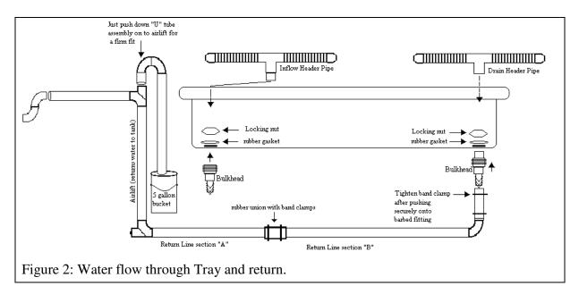
a) The end of the Aquaponic Tray you place closest to the fish tank will be the Inflow end. Make sure that both sides of the Inflow hole are completely clean and free from all dirt and debris. Experience shows that even a small particle under a gasket can cause a leak! Check that the other surfaces are clean as well: the area on both sides of the Inflow hole in the Aquaponic Tray and both shoulders of the Inflow Bulkhead Assembly.
