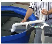
Figure 10: Aim water outlet to encourage circular flow
