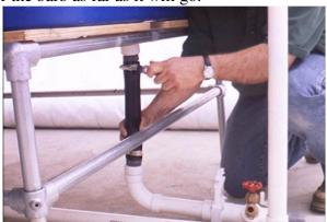
Lubricate the tip of the gray barb coming down from the Inflow Bulkhead Assembly with a smear of sealant.
