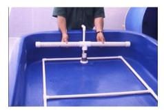
Figure 8: The Air Ring and Inflow Header go into the Tray
