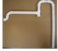
Completed Airlift Water Pump Assembly
