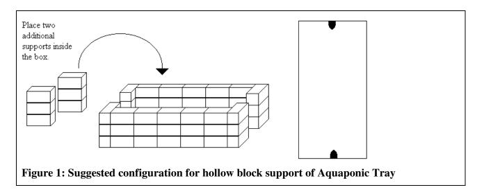
The final height of a stand should be about 24 1/2" when level; it should measure 48" wide and 96" long on the outside dimensions. However, ideally, the Aquaponic Tray should rest about 2 inches higher (no more than three to four inches) at the end closest to the fish Tank. This is to facilitate gravity-assisted water movement through the Tray, and will optimize the overall function of the system. Should you decide to incorporate a
