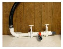
Valve Assembly (Gate and Ball Valves)
