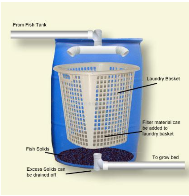
Figure 23. A simplistic drum filter, where water enters at the top and the water sent to the grow beds comes out through the center of the inner basket [40]
