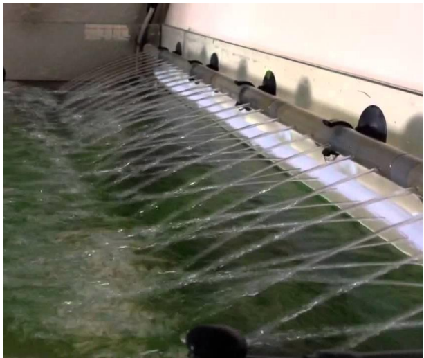
Figure 18. A spray bar accomplishing aeration and degasification [36]
