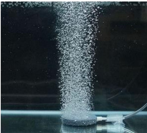
Figure 15. An air stone accomplishing aeration and degasification [33]
