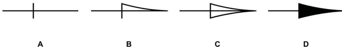
Figure 2-30 — Method of drawing an arrowhead.
