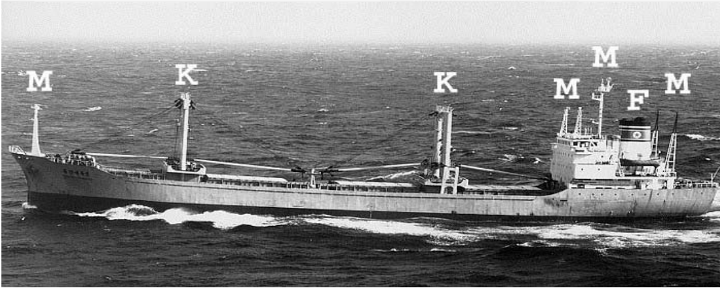
Figure 11-14: Coding of uprights.
