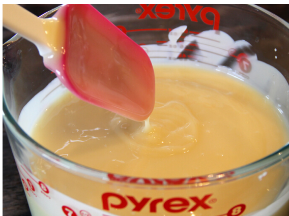
The soap has traced. You can visually see soap sit on the surface of the mixture when drizzled off a spatula or stick blender.
