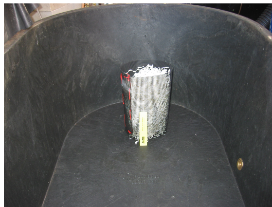
Figure 8. Plastic fish tanks with biofilter. A 15 cm ruler is shown for size reference.
