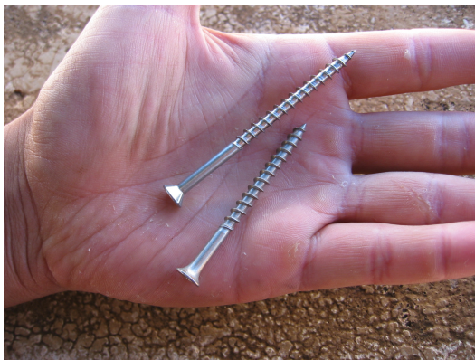
Figure 2. Steel screws used to attach the walls of the grow-beds.
