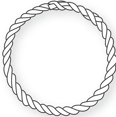
Making Rope Grommets can help you better understand the structure of three-strand rope. Because synthetic rope tends to forget its shape when unlayed, it is awkward to use for making a Grommet.
