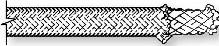
**FIGURE 2-2:** Structure of braid-on-braid rope
