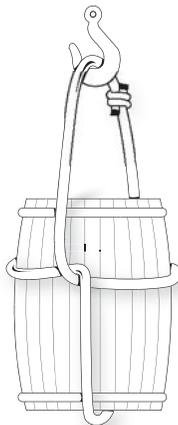
Make sure that the sling is symmetrical on the barrel before lifting.
