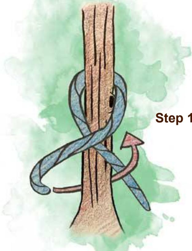
The Constrictor Knot is one of the most secure, but difficult to untie knots. Especially after a load has been applied to this knot, it may become so difficult to untie that it must be cut to release it.
