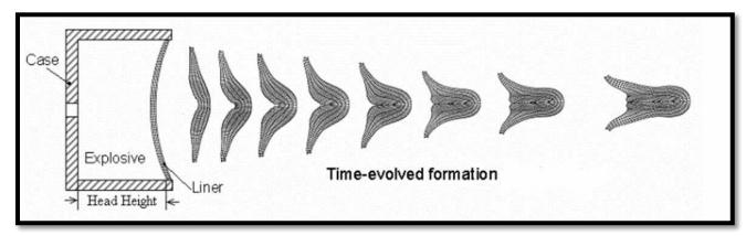
Figure 51 (U) Generic Explosively Formed Penetrator Warhead Design
