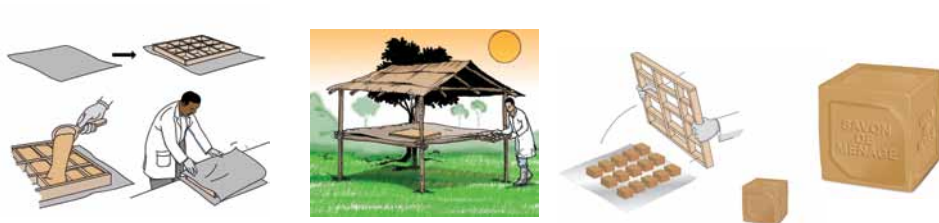
⬆️ Moulding the soap, drying it and removing it from the mould
