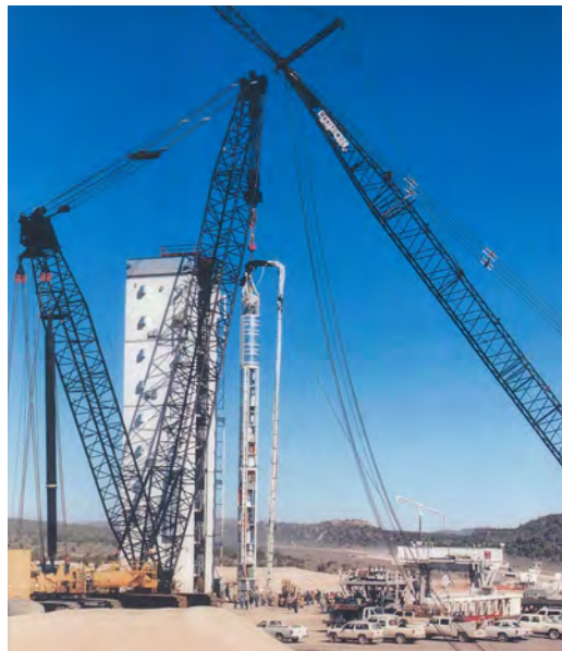
Barnwell was a test conducted on December 8, 1989, underground at Pahute Mesa on the NNSS. Barnwell was a Joint US-UK test with a yield of 20 to 150 kt. Shown at right is the diagnostic rack ready for lowering down the emplacement hole.
