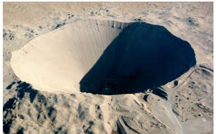
Sedan crater was formed when a 104-kt explosion buried under 635 ft of desert alluvium was fired at the NNSS on July 6, 1962, displacing 12 million tons of earth. The crater is 320 ft deep and 1,280 ft in diameter.
