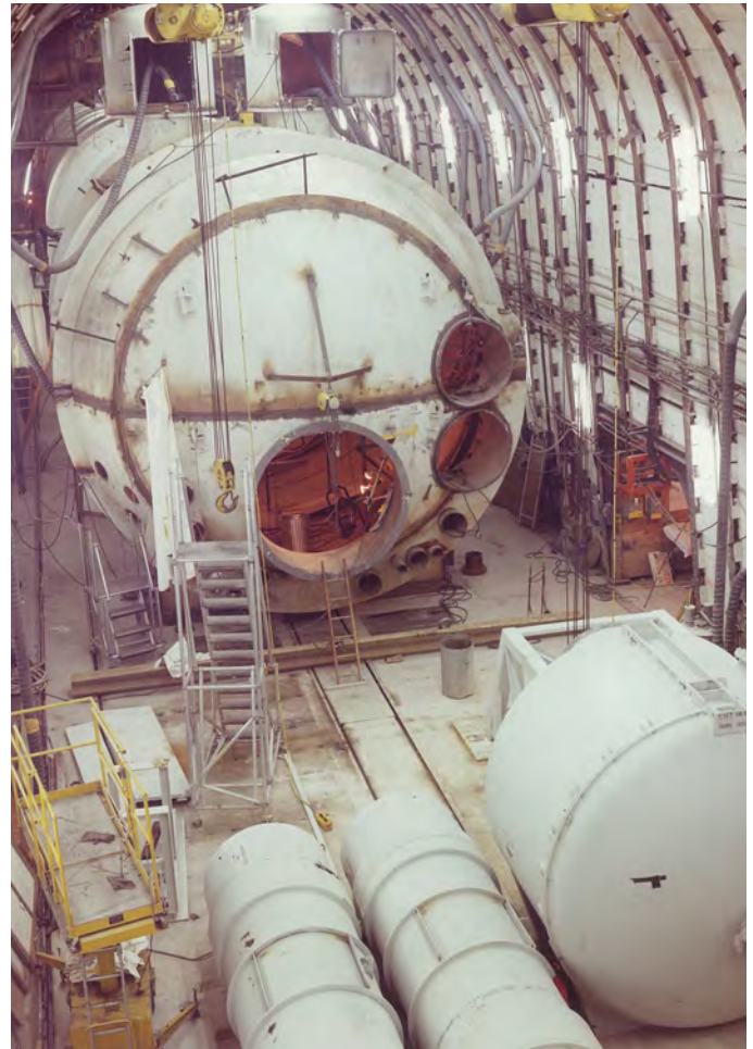
Diamond Sculls was a test conducted on July 20, 1972, in a tunnel at Rainier Mesa on the NNSS. Diamond Sculls was a weapons effects test where the radiation from the detonation traveled 2,000 ft down a tapered horizontal line-of-sight pipe to the test chambers (shown above), which were 27 ft in diameter. Fast-closure doors in the pipe stopped flying debris after the radiation went by and protected the experiments from debris-impact damage.
