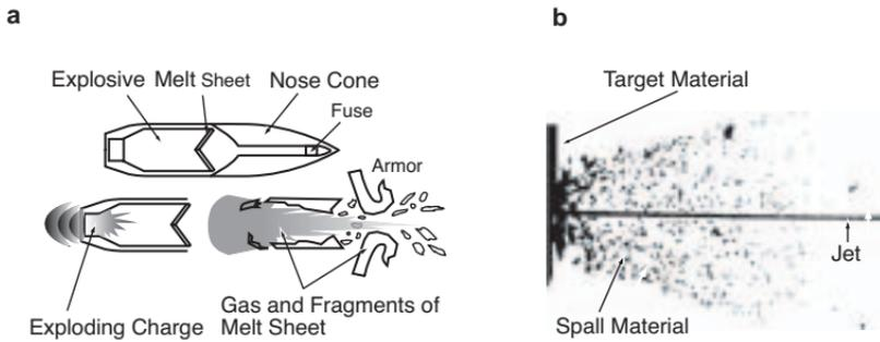
**Fig. 1-7.** (a) Disruptive mechanisms of the shaped-charge warhead, (b) diagram taken from photograph of an actual detonation of shaped-charged warhead against armor plate caused by antitank land mines.
