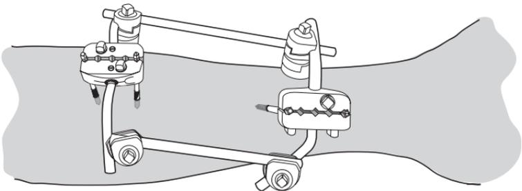
**Fig. 23-23.** Two-bar apparatus. As the majority of tibia fractures are unstable, it creates a more stable construct by adding a second bar. This requires the use of two of the kits but makes little difference when you are using the tub container at the CSH or equivalent hospitals.
