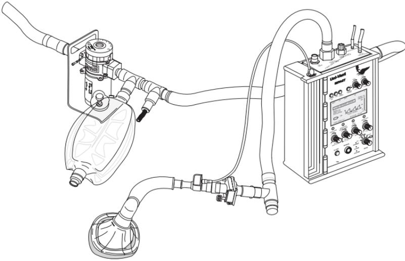
Fig. 9-1. Draw-over apparatus in combination with the ventilator.
