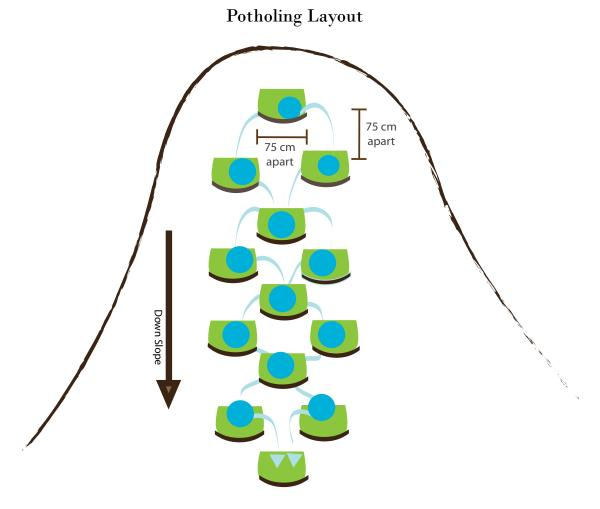
Figure 4.2 Layout of a pothole field
