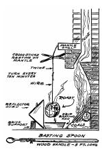
Roast beef, either rib or rolled, needs constant turning before a reflector fire. Bind the roast with stovepipe wire, both ways, to hold it tightly together. Have one lead wire running up from the roast and fasten to a piece twine or cord. This to provide for twisting. Fasten twine to top of fireplace shelf
