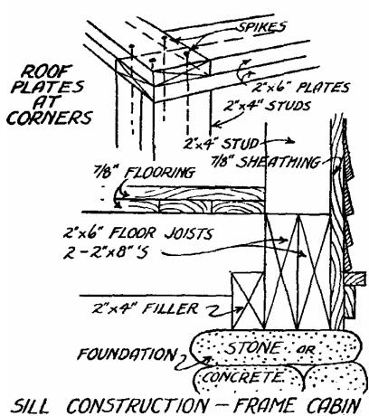
Here we have plates at top of studding fastened at corners, also sill construction on foundation. To keep your cabin warm underfoot it is build well to double floor filled in between with tar paper.
